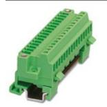
DIN rail connector, nominal current: 8 A, number of positions: 6, pitch: 3.81 mm, connection method: Screw connection with tension sleeve, color: green, contact surface: Tin, mounting: DIN rail
