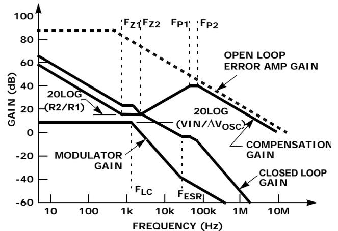
FIGURE 18. ASYMPTOTIC BODE PLOT OF CONVERTER GAIN
