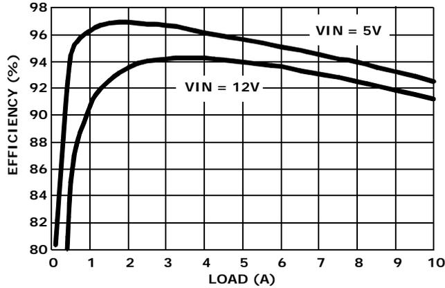
FIGURE 7. EFFICIENCY vs LOAD CURRENT ( $V_{OUT} = 3.3V$ )
