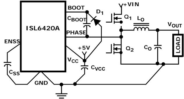
FIGURE 16. PRINTED CIRCUIT BOARD SMALL SIGNAL LAYOUT GUIDELINES
