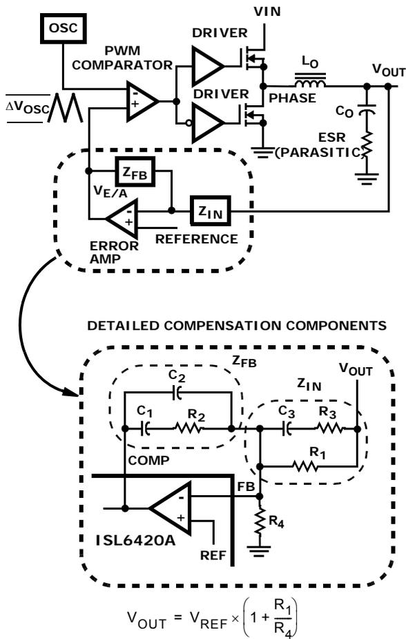
FIGURE 17. VOLTAGE - MODE BUCK CONVERTER COMPENSATION DESIGN
