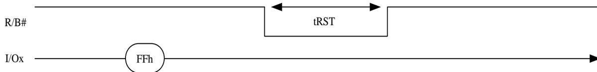
**Figure 8.10 Reset Operation**
