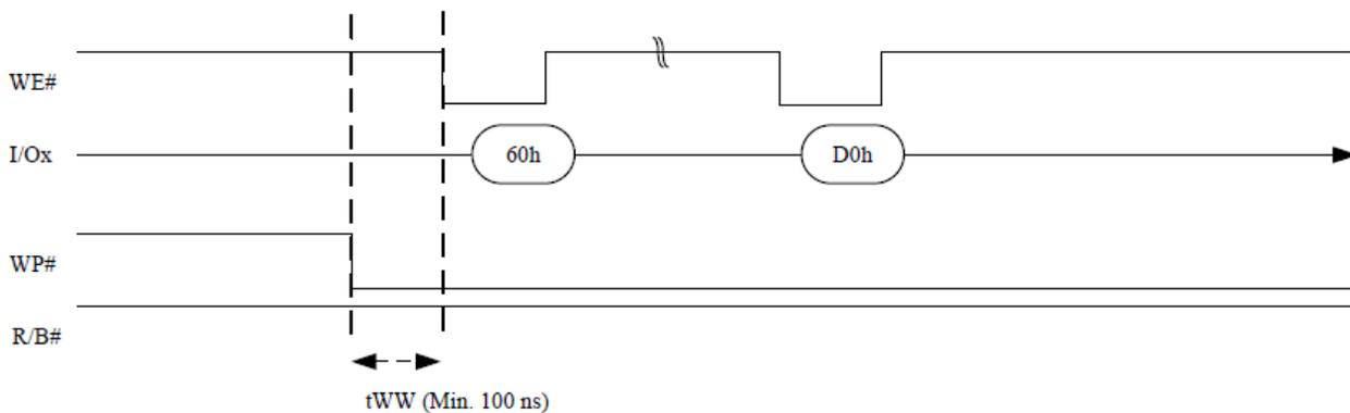
Figure 8.14 Enable/Disable Programming and Enable Erasing
