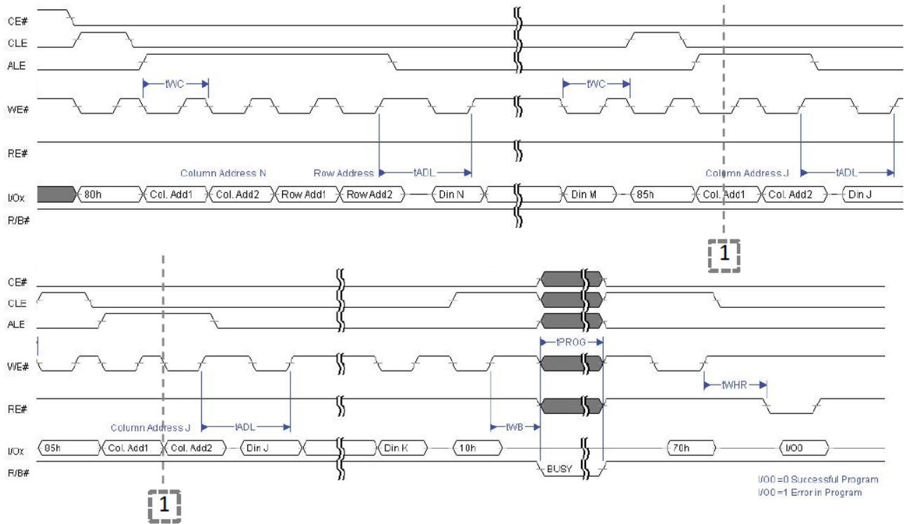
**Note:** t<sub>ADL</sub> is the time from the WE# rising edge of final address cycle to the WE# rising edge of the first data cycle.
