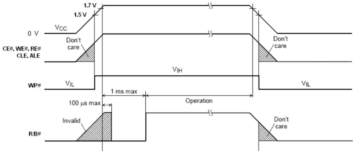
**Figure 8.13 AC Waveforms for Power Transition**
