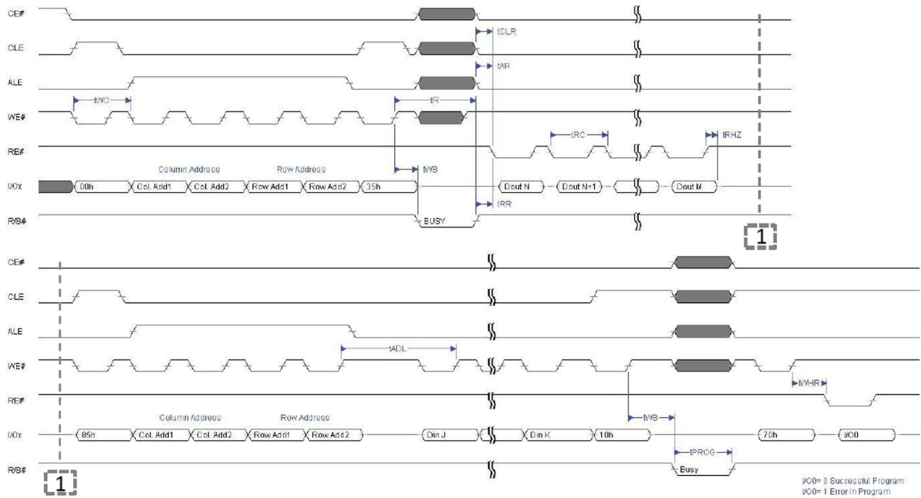
**Figure 6.12 Copy-Back Operation with Random Data Input**
