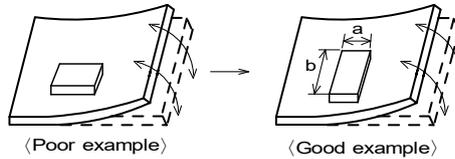
(2) Components location on PCB separation
