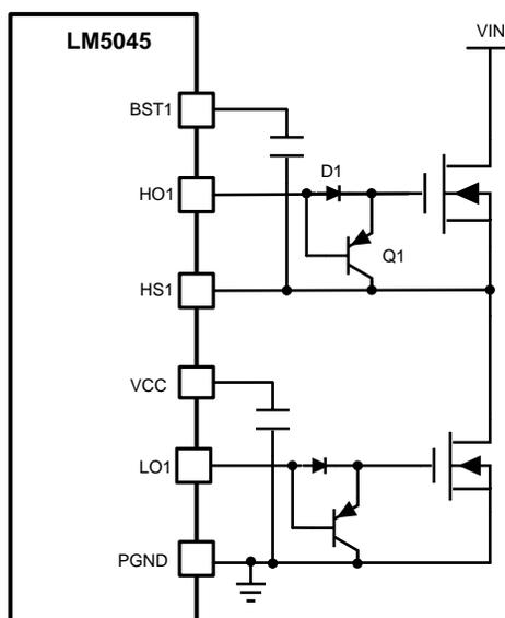
Figure 30. Circuit to Speed-Up the Turnoff Process
