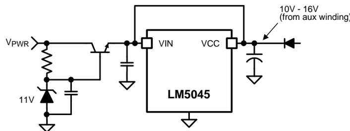
**Figure 21. Start-Up Regulator For  $V_{PWR} > 100$  V**
