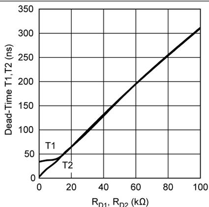
Figure 7. Dead-Time T1, T2 vs  $R_{D1}, R_{D2}$
