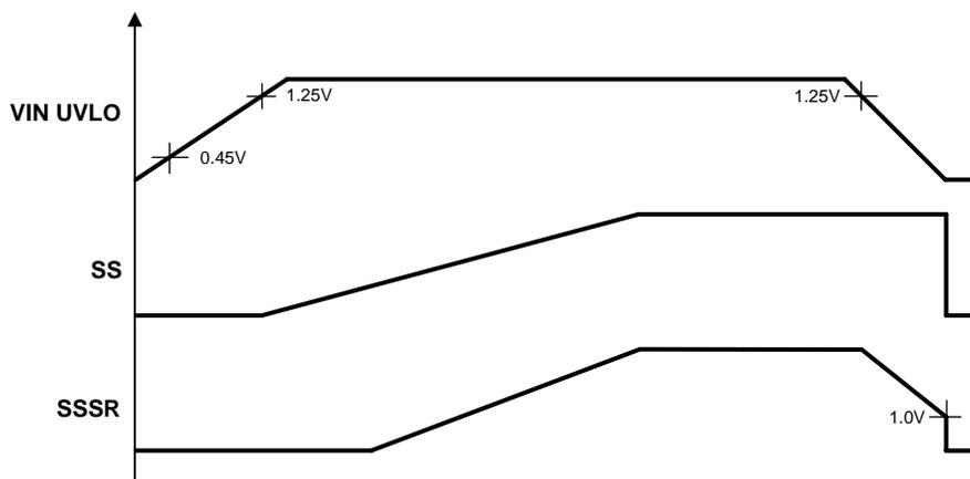
Figure 16. Stop-Stop Waveforms During a UVLO Event
