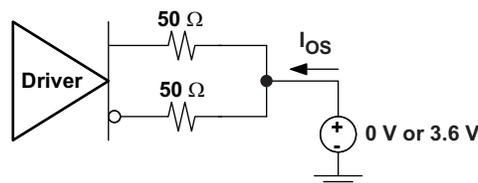
Figure 20. TMDS Main Link Short Circuit Output Circuit
