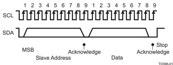
Figure 41. I<sup>2</sup>C Address, Data Cycle(s), and Stop
