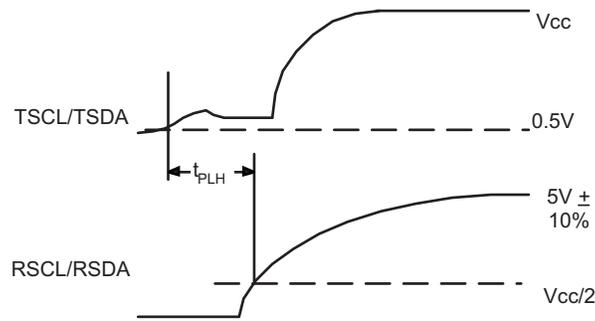
Figure 33. Waveform of Driver T Turning Off
