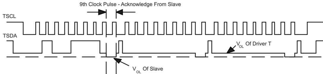
Figure 36. Bus T Waveform
