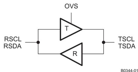
**Figure 32. I<sup>2</sup>C Drivers in the TMDS461 = Side Is the HDMI Source Side, T Side Is the HDMI Sink Side)**
