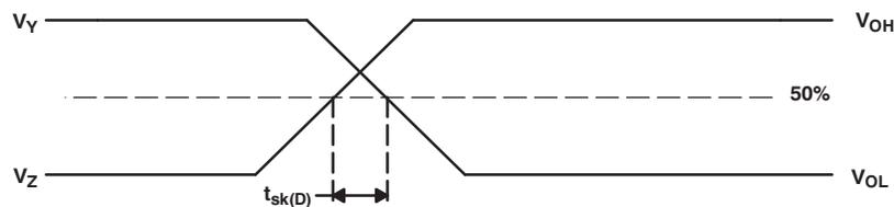
Figure 15. Definition of Intra-Pair Differential Skew
