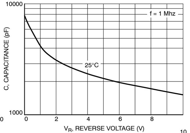
Figure 4. Typical Capacitance
