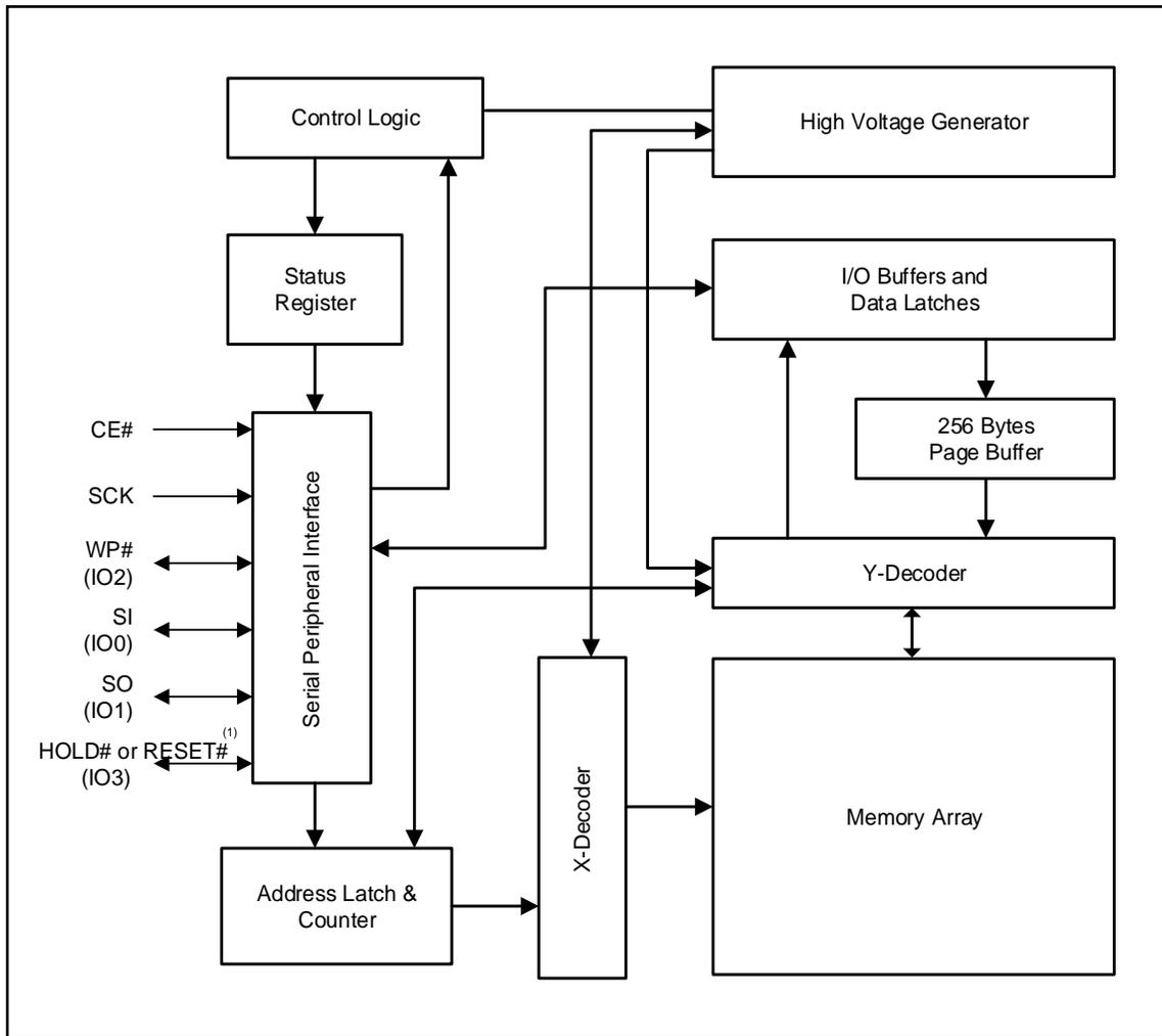
**Note1:** For RESET# (IO3) pin option instead of HOLD# (IO3) pin, call Factory. In case of device with dedicated RESET# function, RESET# is on pin3/ball A4. See the Ordering Information for the dedicated RESET# option.
