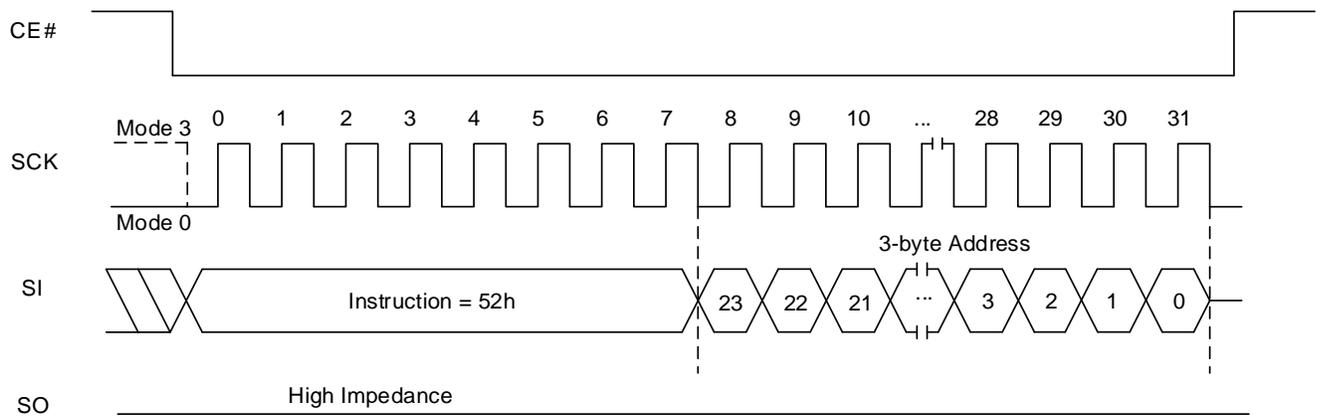
**Figure 8.19 Block Erase (32K) QPI Sequence**
