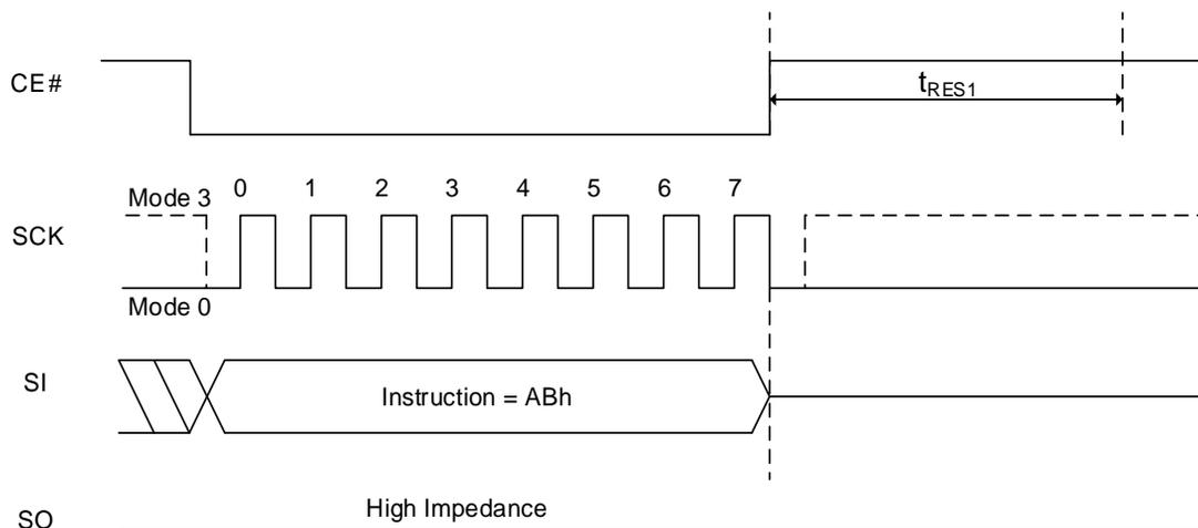
**Figure 8.39 Release Power Down QPI Sequence**
