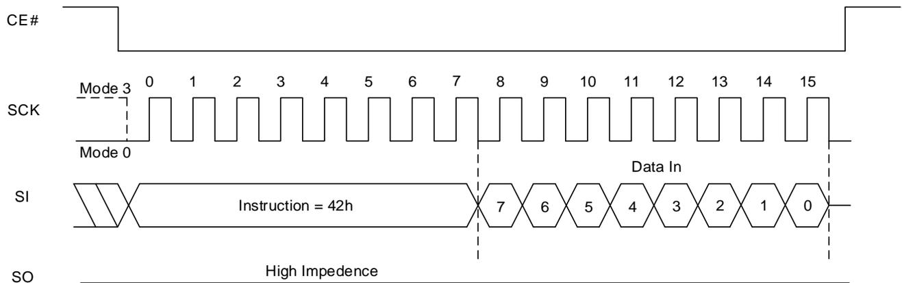
**Figure 8.33 Write Function Register QPI Sequence**
