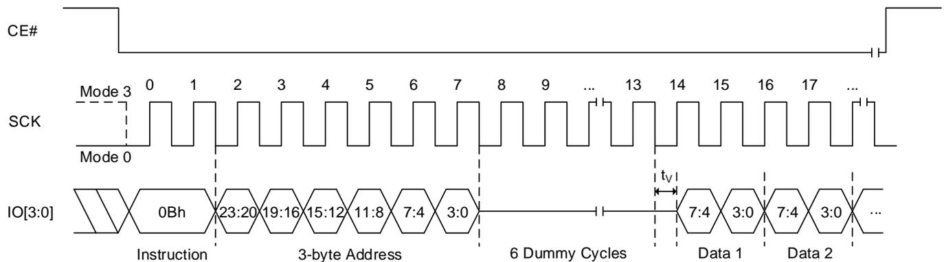
**Note: Number of dummy cycles depends on Read Parameter setting. Detailed information in Table 6.10 Read Dummy Cycles.**
