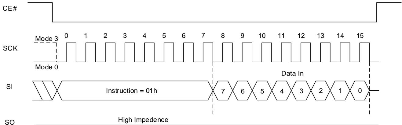
**Figure 8.29 Write Status Register QPI Sequence**
