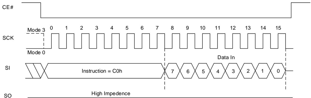
**Figure 8.41 Set Read Parameters QPI Sequence**
