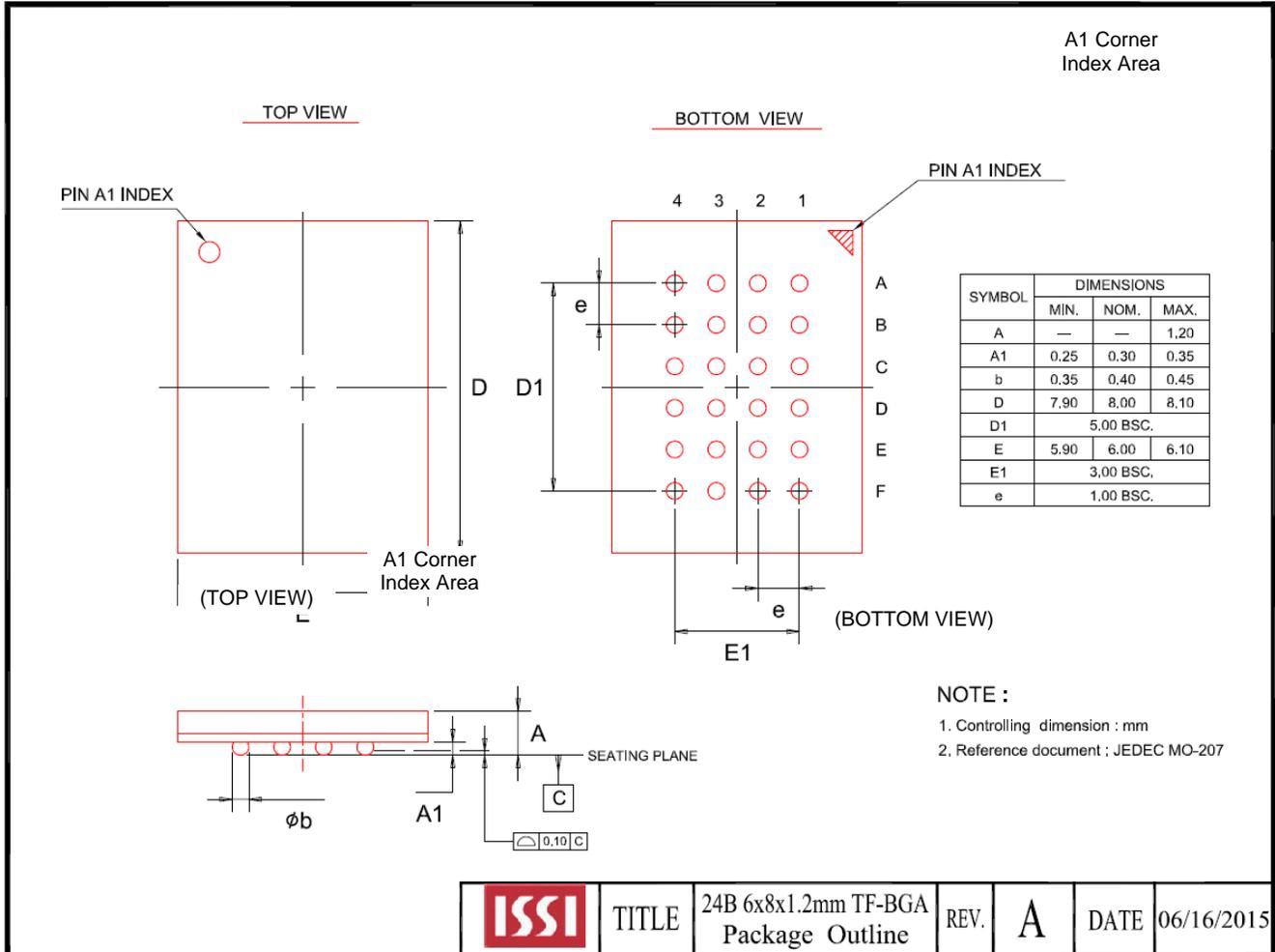
**10.7 24-BALL THIN PROFILE FINE PITCH BGA 6X8MM 5X5 BALL ARRAY (H)**
