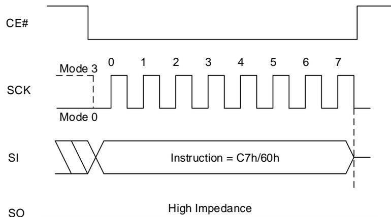
**Figure 8.21 Chip Erase QPI Sequence**
