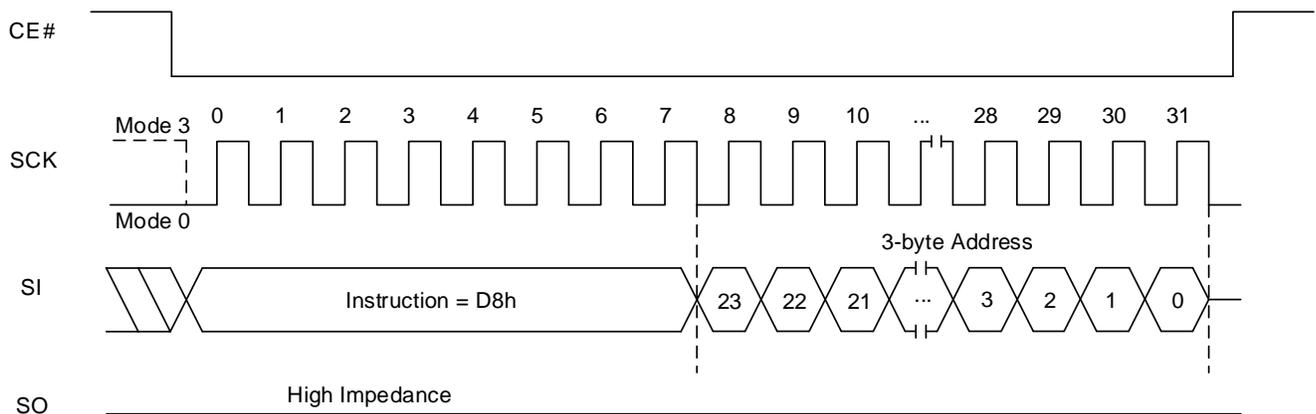
**Figure 8.17 Block Erase (64K) QPI Sequence**
