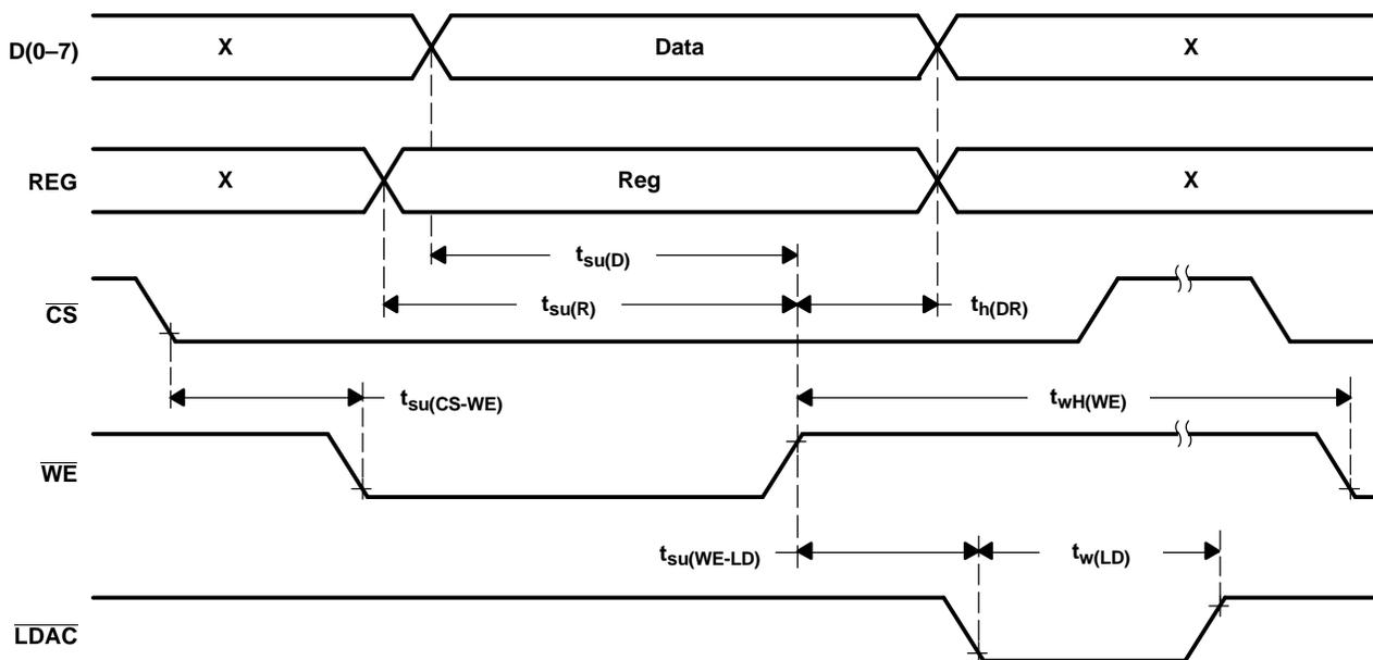
**Figure 1. Timing Diagram**
