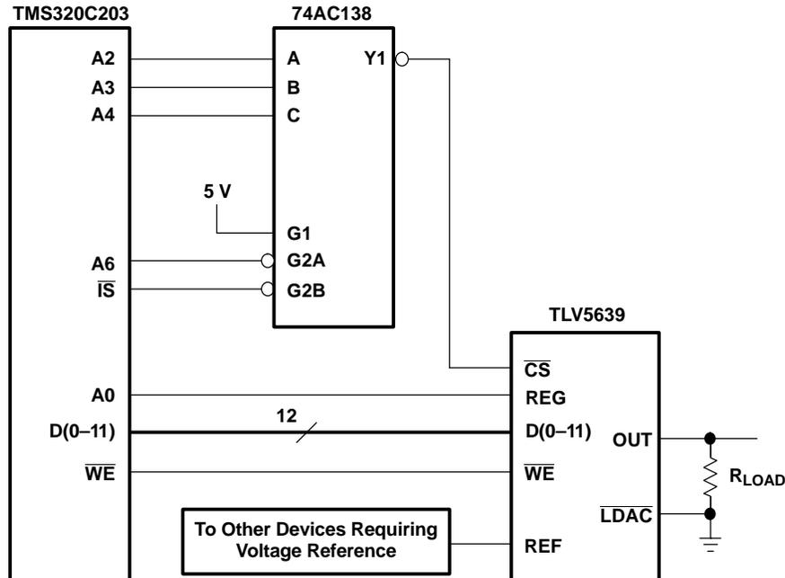
Figure 13. TLV5639 to TMS320C203 DSP Interface Connection
