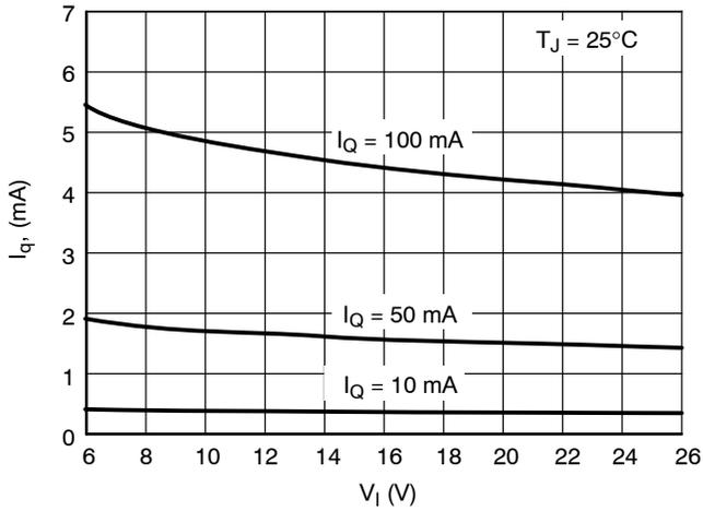
Figure 16. Current Consumption  $I_q$  vs. Input Voltage  $V_I$
