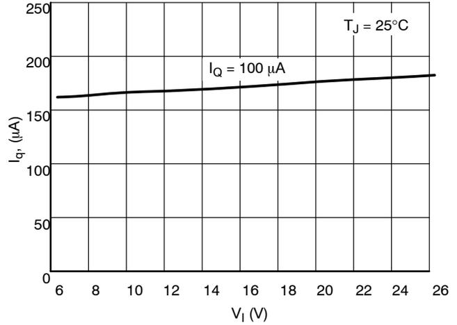
Figure 17. Current Consumption  $I_q$  vs. Input Voltage  $V_I$
