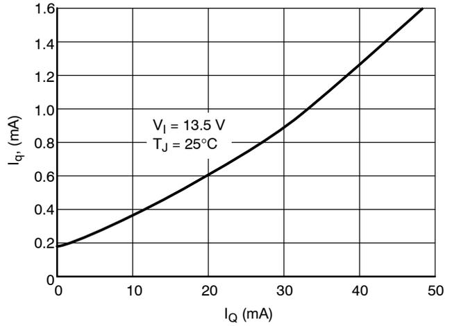
Figure 15. Current Consumption  $I_q$  vs. Output Current  $I_Q$
