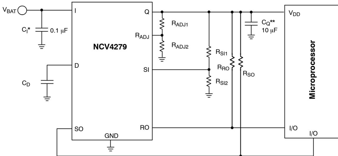
\* $C_1$  required if regulator is located far from the power supply filter.
