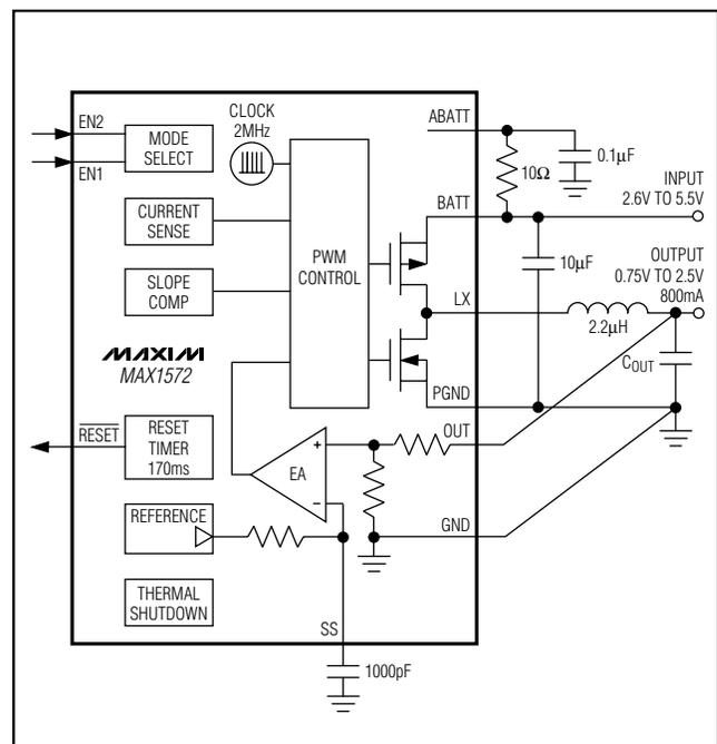
Figure 1. Functional Diagram
