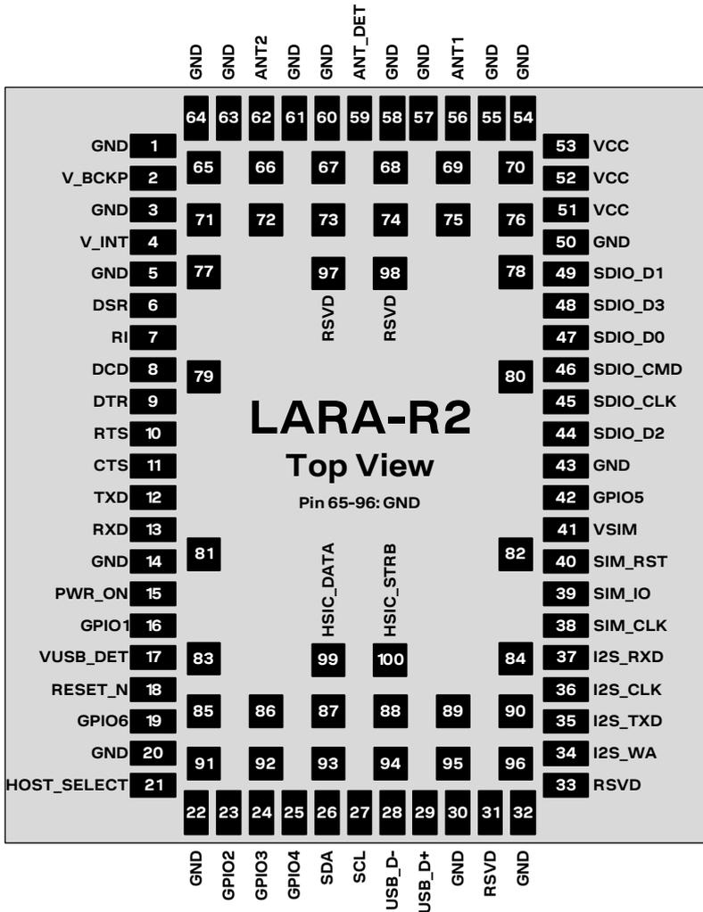
Figure 2: LARA-R2 series pin assignment (top view)
