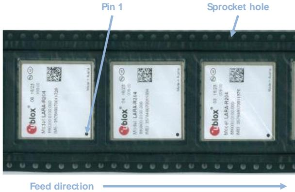
Figure 5: Orientation for LARA-R2 series modules on tape
