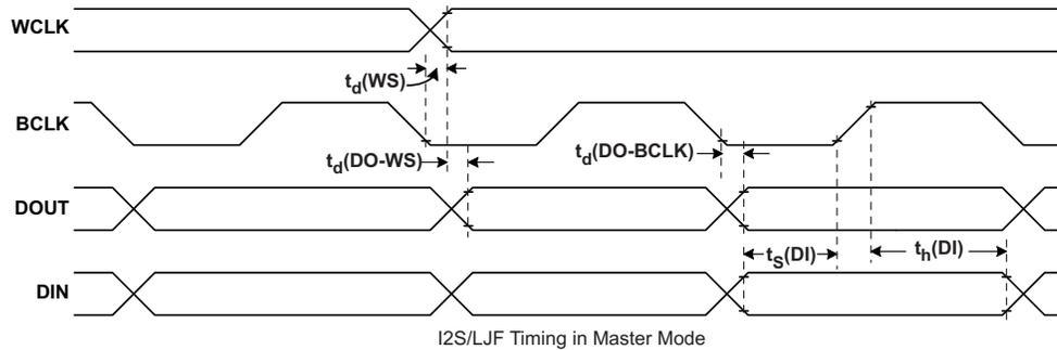
Figure 4. I<sup>2</sup>S/LJF/RJF Timing in Master Mode
