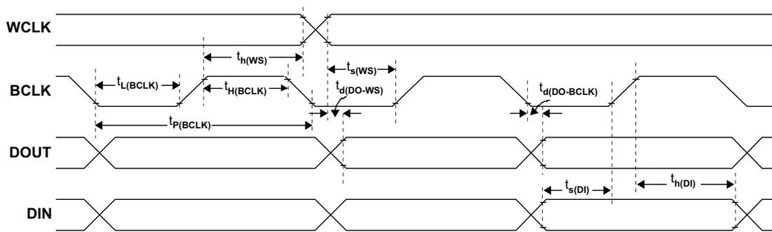
Figure 5. I<sup>2</sup>S/LJF/RJF Timing in Slave Mode
