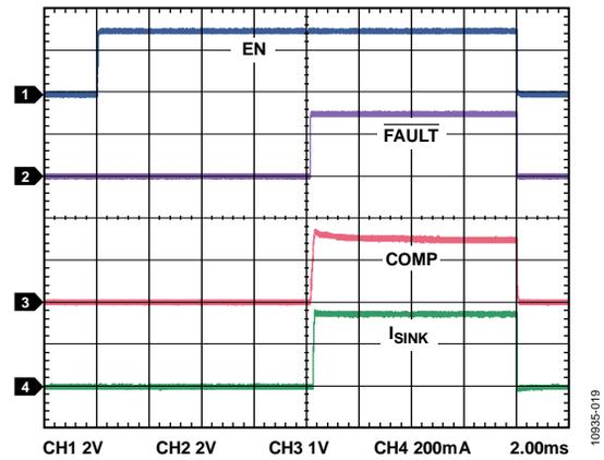
Figure 19. Start-Up Sequence (See Figure 1 Setup)
