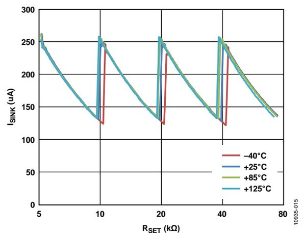
Figure 15. Sink Current vs.  $R_{SET}$  (DIM = 0 V)
