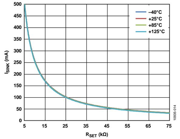
Figure 14. Sink Current vs.  $R_{SET}$  (DIM = 3 V)
