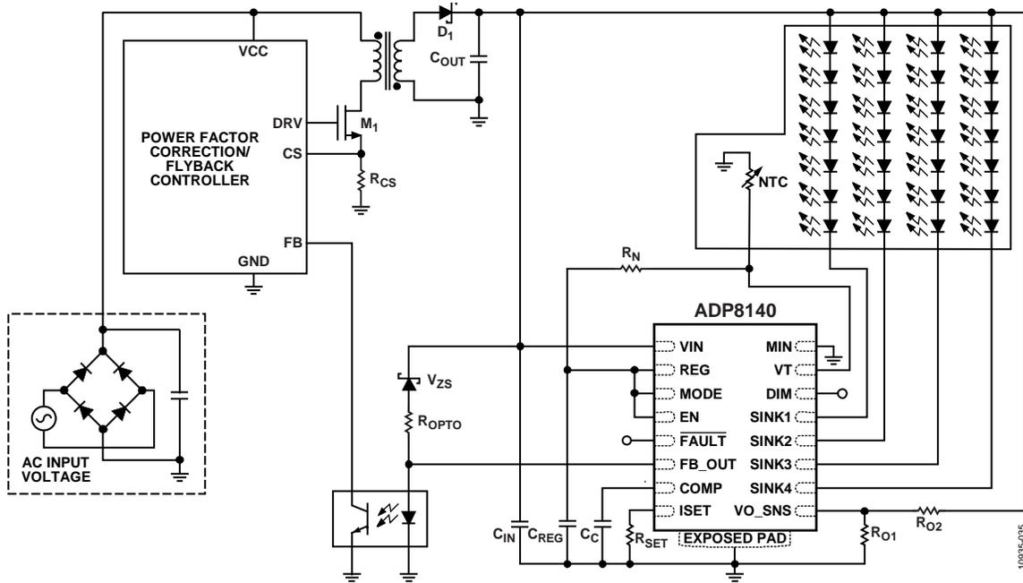
Figure 33. ADP8140 Secondary Side Control Design Example
