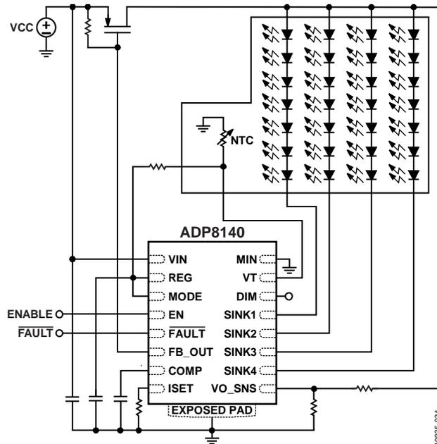
Figure 32. ADP8140 with a PMOS Regulation Stage
