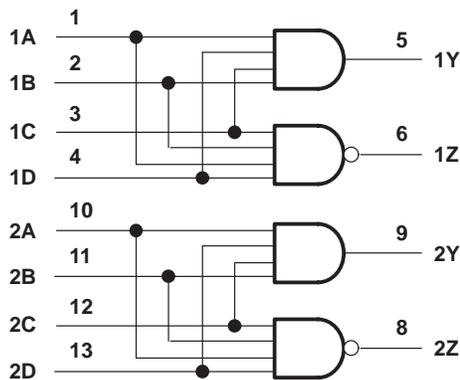
Positive logic:  $y = ABCD$ ,  $Z = \overline{ABCD}$
