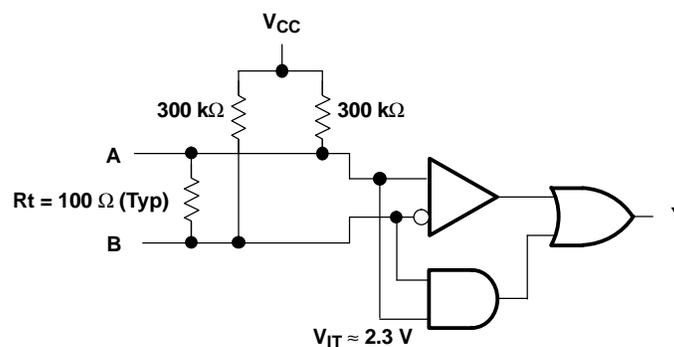
Figure 18. Open-Circuit Fail Safe of the LVDS Receiver
