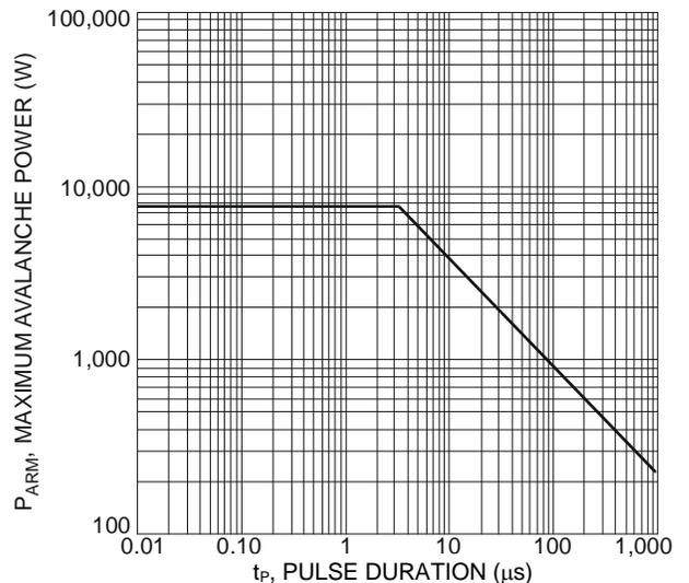
Figure 8 Maximum Avalanche Power Curve, Per Element
