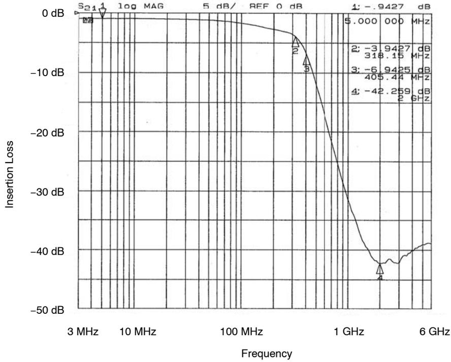
Figure 3. Filter 3 Insertion Loss (CM1461-04DE)
