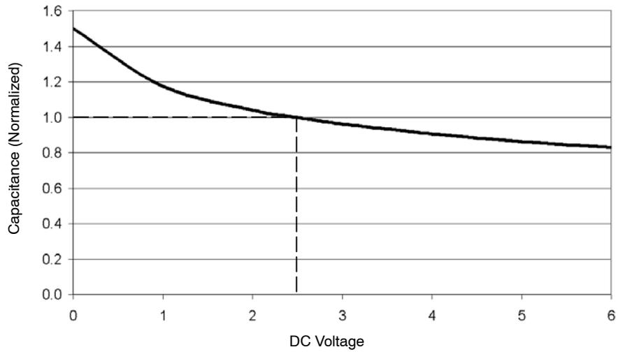
**Figure 19. Filter Capacitance vs. Input Voltage
