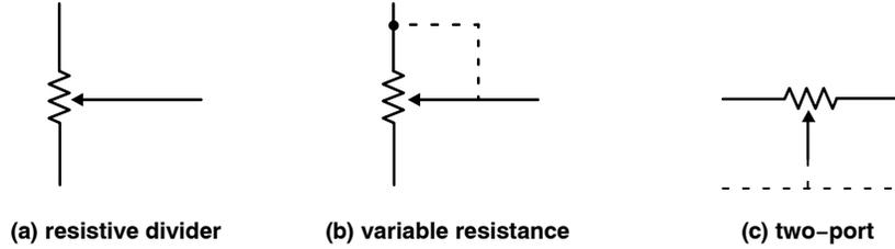
Figure 5. Potentiometer Configuration
