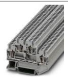
Component terminal block, Connection type: Spring-cage connection, Cross section: 0.08 mm² - 4 mm², AWG: 28 - 12, Nominal current: 22 A, Nominal voltage: 500 V, Length: 67.5 mm, Width: 5.2 mm, Color: black, Assembly: NS 35/7,5, NS 35/15
