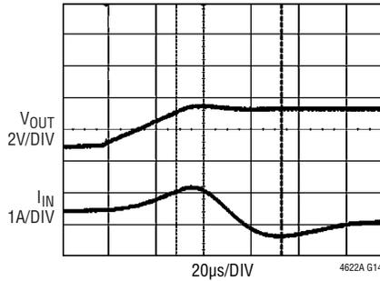
$V_{IN} = 12V$ ,  $V_{OUT} = 3.3V$ ,  $f_{SW} = 1MHz$
