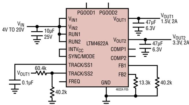
Figure 5. Example Schematic of Ratiometric Output Voltage Tracking
