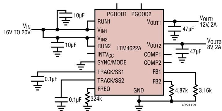
Figure 29. 16V<sub>IN</sub> to 20V<sub>IN</sub>, 12V and 8V Output at 2A with 2MHz Switching Frequency
