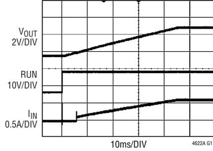
$V_{IN} = 12V$ ,  $V_{OUT} = 3.3V$ ,  $f_{SW} = 1MHz$
