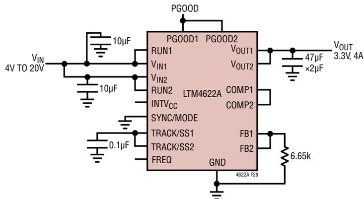
Figure 28. 4V<sub>IN</sub> to 20V<sub>IN</sub>, 3.3V Two Phase in Parallel 4A Design
