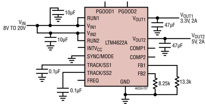
Figure 27. 8V<sub>IN</sub> to 20V<sub>IN</sub>, 3.3V and 5V Output at 2A Design
