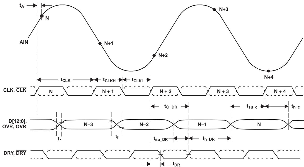
Figure 2. Timing Diagram
