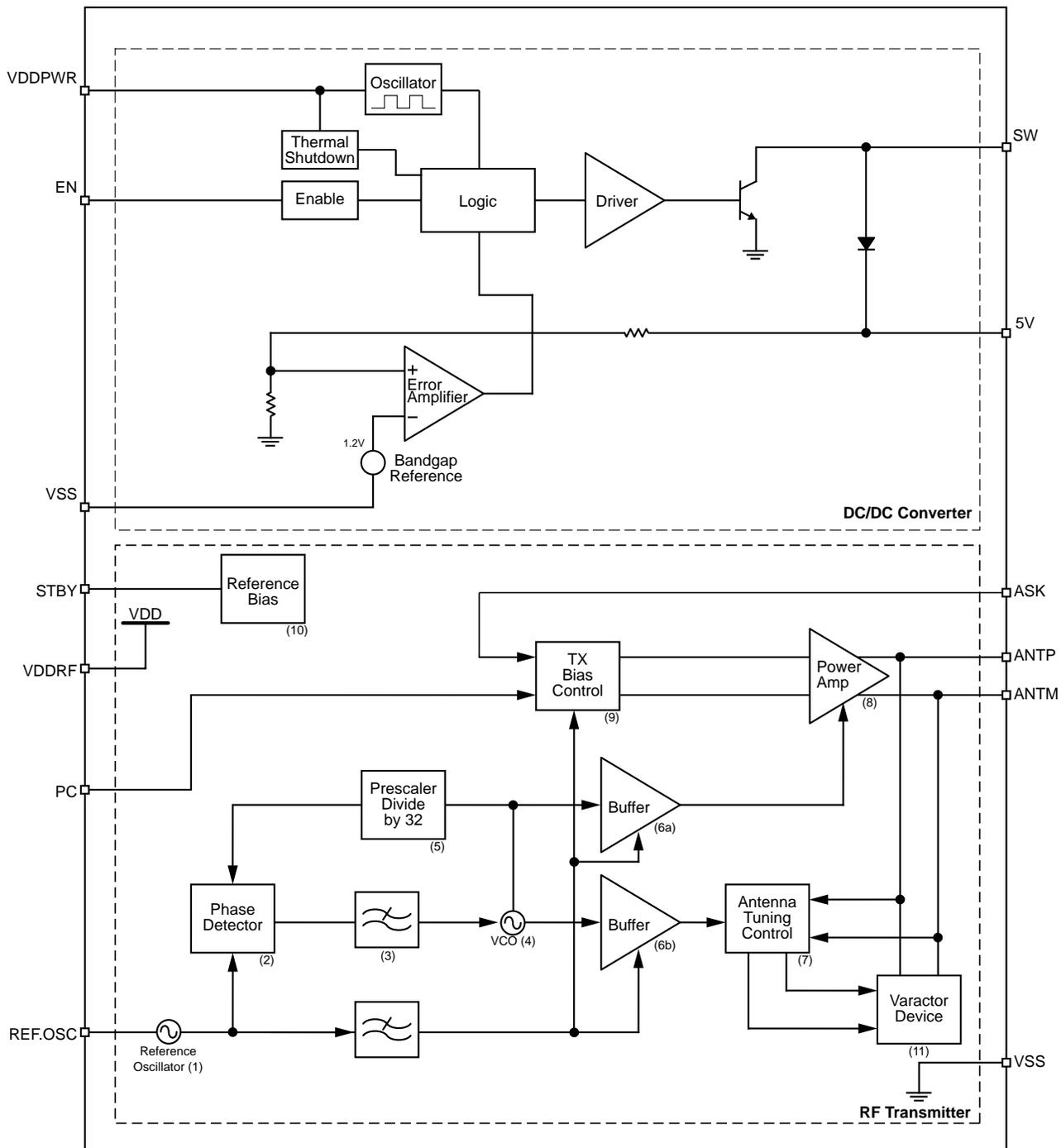
Figure 2. MICRF104 Block Diagram (RF Circuit)
