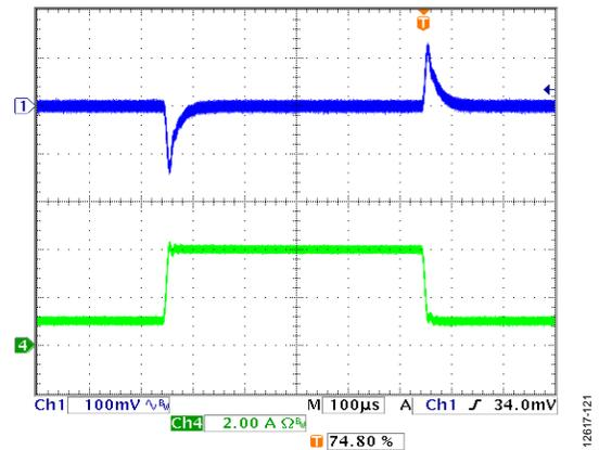
Figure 21. Channel 1/Channel 2 Load Transient, 1 A to 4 A,  $V_{IN} = 12\text{ V}$ ,  $V_{OUT} = 3.3\text{ V}$ ,  $f_{SW} = 600\text{ kHz}$ ,  $L = 2.2\text{ }\mu\text{H}$ ,  $C_{OUT} = 47\text{ }\mu\text{F} \times 2$ , Channel 1 =  $V_{OUTx}$ , Channel 4 =  $I_{OUTx}$
