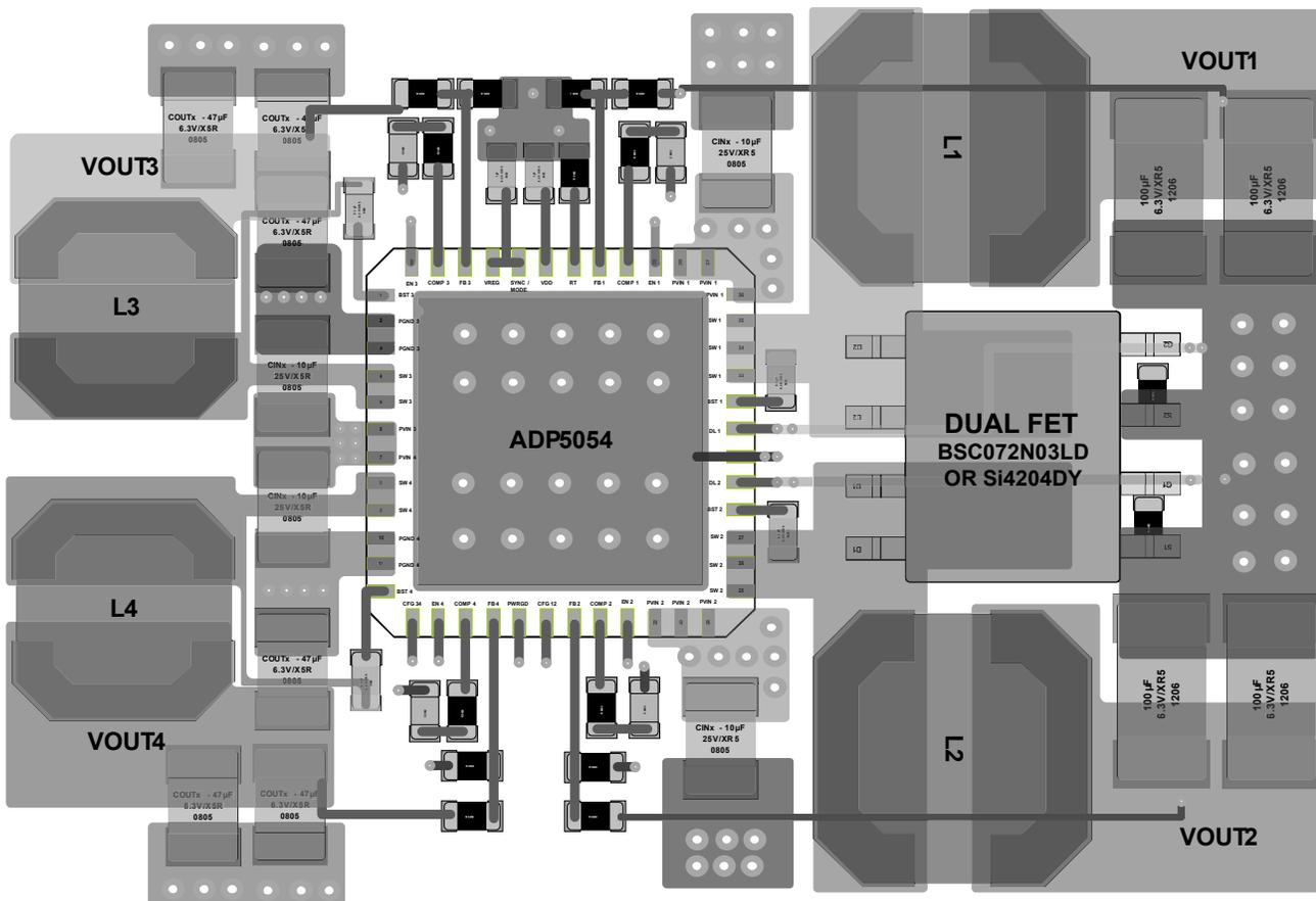
Figure 43. Typical PCB Layout for the ADP5054
