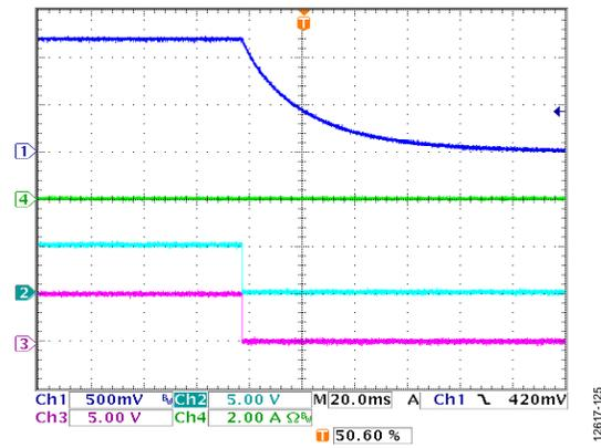
Figure 25. Channel 1 Shutdown with Active Output Discharge,  $V_{IN} = 12\text{ V}$ ,  $V_{OUT} = 1.2\text{ V}$ ,  $f_{SW} = 600\text{ kHz}$ ,  $L = 1\text{ }\mu\text{H}$ ,  $C_{OUT} = 47\text{ }\mu\text{F} \times 2$ , Channel 1 =  $V_{OUT1}$ , Channel 2 = EN1, Channel 3 = PWRGD, Channel 4 =  $I_{OUT1}$
