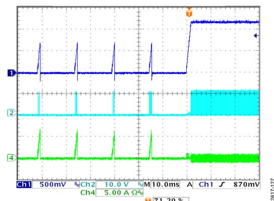
Figure 27. Short-Circuit Protection Recovery,  $V_{IN} = 12\text{ V}$ ,  $V_{OUT} = 1.2\text{ V}$ ,  $f_{SW} = 600\text{ kHz}$ ,  $L = 1\text{ }\mu\text{H}$ ,  $C_{OUT} = 47\text{ }\mu\text{F} \times 2$ , Channel 1 =  $V_{OUTX}$ , Channel 2 = SWX, Channel 4 =  $I_{LX}$
