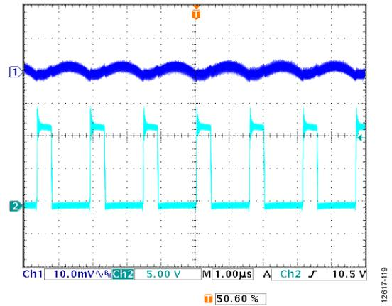
Figure 19. Steady State Waveform at Heavy Load,  $V_{IN} = 12\text{ V}$ ,  $V_{OUT} = 3.3\text{ V}$ , Output Load Current ( $I_{OUT}$ ) = 3 A,  $f_{SW} = 600\text{ kHz}$ ,  $L = 4.7\text{ }\mu\text{H}$ ,  $C_{OUT} = 47\text{ }\mu\text{F} \times 2$ , FPWM Mode, Channel 1 =  $V_{OUTx}$ , Channel 2 =  $SWx$
