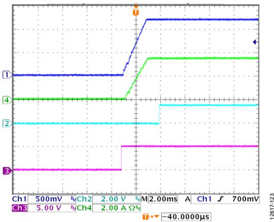
Figure 23. Channel 1 Soft Start with 4 A Resistance Load,  $V_{IN} = 12\text{ V}$ ,  $V_{OUT} = 1.2\text{ V}$ ,  $f_{SW} = 600\text{ kHz}$ ,  $L = 1\text{ }\mu\text{H}$ ,  $C_{OUT} = 47\text{ }\mu\text{F} \times 2$ , Channel 1 =  $V_{OUT1}$ , Channel 2 = PWRGD, Channel 3 = EN1, Channel 4 =  $I_{OUT1}$
