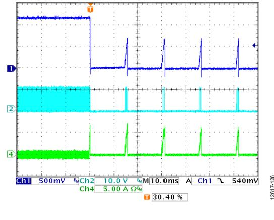
Figure 26. Short-Circuit Protection Entry,  $V_{IN} = 12\text{ V}$ ,  $V_{OUT} = 1.2\text{ V}$ ,  $f_{SW} = 600\text{ kHz}$ ,  $L = 1\text{ }\mu\text{H}$ ,  $C_{OUT} = 47\text{ }\mu\text{F} \times 2$ , Channel 1 =  $V_{OUTX}$ , Channel 2 = SWX, Channel 4 =  $I_{LX}$
