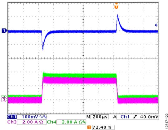
Figure 22. Load Transient, Channel 1/Channel 2 Parallel Output, 0 A to 6 A,  $V_{IN} = 12\text{ V}$ ,  $V_{OUT} = 3.3\text{ V}$ ,  $f_{SW} = 600\text{ kHz}$ ,  $L = 4.7\text{ }\mu\text{H}$ ,  $C_{OUT} = 47\text{ }\mu\text{F} \times 4$ , Channel 1 =  $V_{OUT}$ , Channel 3 =  $I_{L1}$ , Channel 4 =  $I_{L2}$
