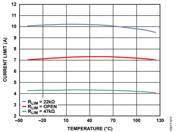
Figure 17. Channel 1/Channel 2 Current Limit vs. Temperature
