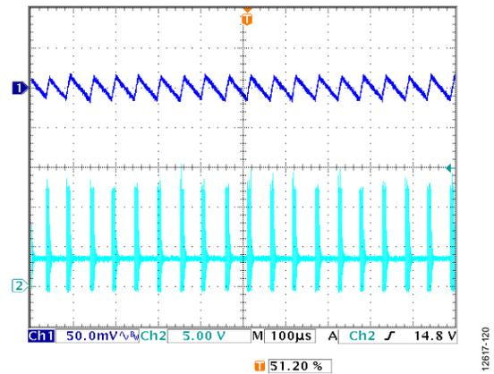
Figure 20. Steady State Waveform at Light Load,  $V_{IN} = 12\text{ V}$ ,  $V_{OUT} = 3.3\text{ V}$ ,  $I_{OUT} = 30\text{ mA}$ ,  $f_{SW} = 600\text{ kHz}$ ,  $L = 4.7\text{ }\mu\text{H}$ ,  $C_{OUT} = 47\text{ }\mu\text{F} \times 2$ , Automatic PWM/PSM Mode, Channel 1 =  $V_{OUTx}$ , Channel 2 =  $SWx$
