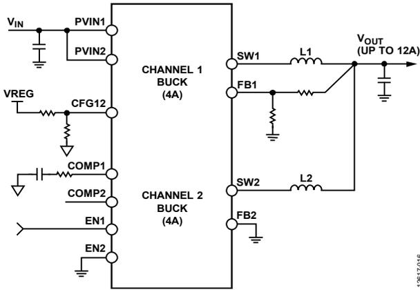
Figure 35. Parallel Operation for Channel 1 and Channel 2
