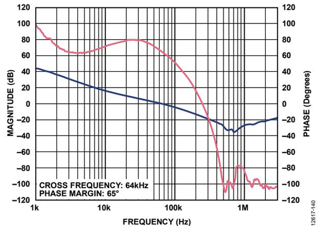
Figure 40. Bode Plot for 1.2 V Output
