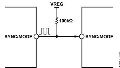
Figure 32. Two ADP5054 Devices Configured for Synchronization Mode
