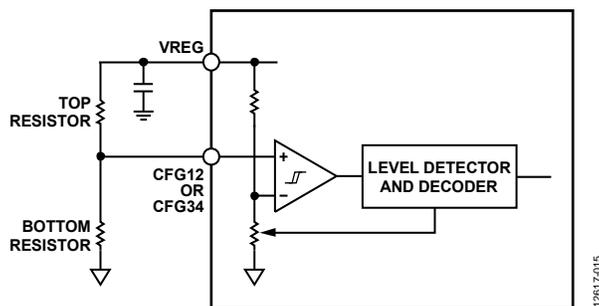
Figure 34. Level Detector Circuit for Soft Start
