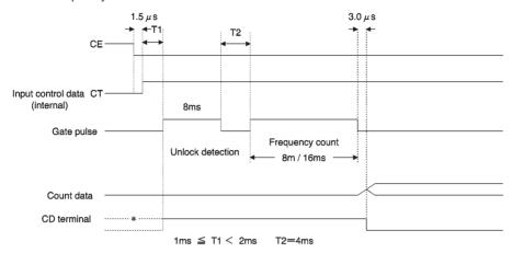
(2) When CT = 0 and GT = 1: Only unlock detection is carried out.
