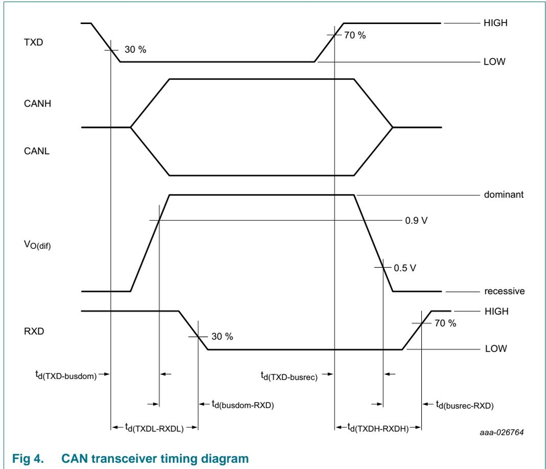
Fig 4. CAN transceiver timing diagram
