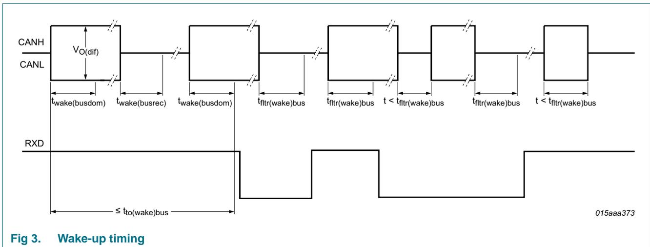
Fig 3. Wake-up timing
