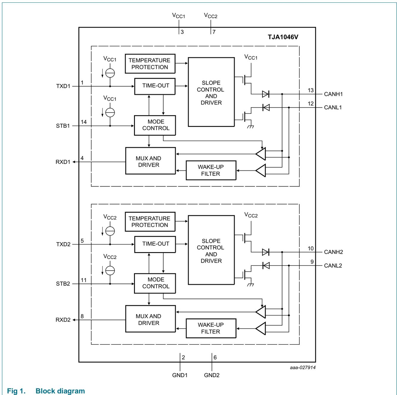
Fig 1. Block diagram
