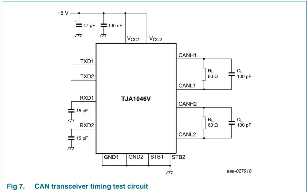
Fig 7. CAN transceiver timing test circuit
