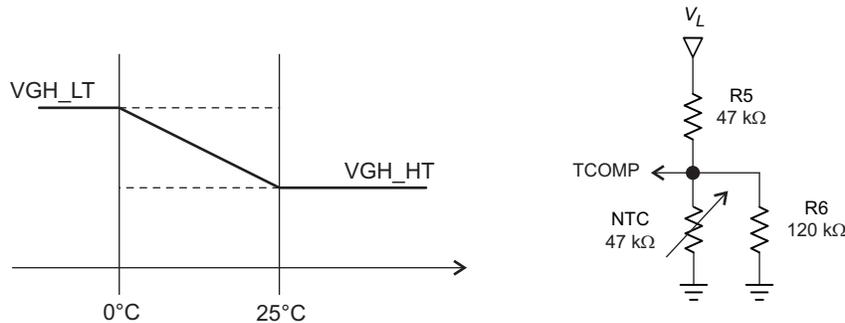
**Setting the output voltage  $V_{GH\_LT}$  and  $V_{GH\_HT}$**
