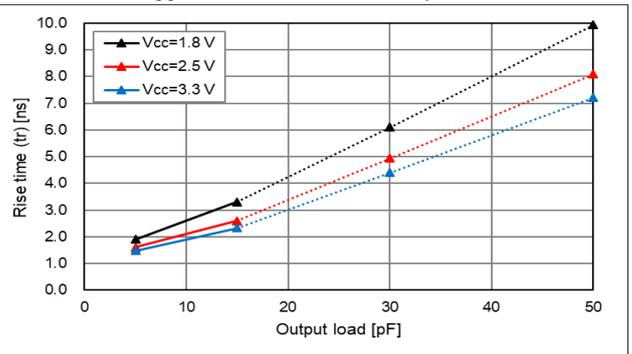
\* Output load condition under L<sub>CMOS</sub> > 15 pF (dotted line area) is not guaranteed, and the data is for reference.
