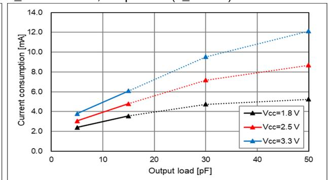
\* Output load condition under  $L_{CMOS} > 15\text{ pF}$  (dotted line area) is not guaranteed, and the data is for reference.
