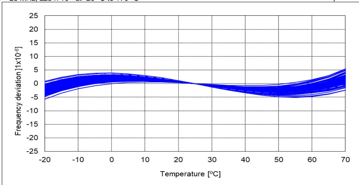
$f_0 = 25 \text{ MHz}$ ,  $\pm 50 \times 10^{-6}$  at  $-40 \text{ }^\circ\text{C}$  to  $+85 \text{ }^\circ\text{C}/+105 \text{ }^\circ\text{C}$
