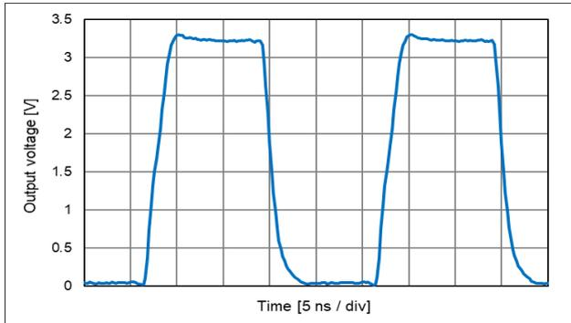
V<sub>CC</sub> = 2.5 V, L<sub>CMOS</sub> = 15 pF, T<sub>use</sub> = +25 °C
