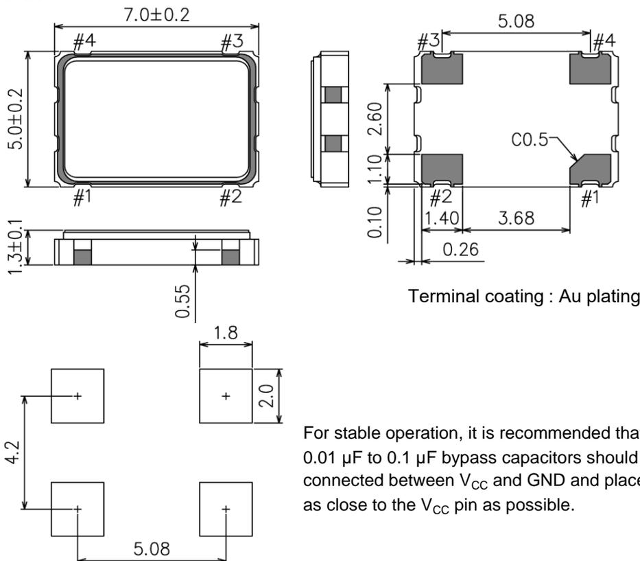
For stable operation, it is recommended that 0.01 μF to 0.1 μF bypass capacitors should be connected between V<sub>CC</sub> and GND and placed as close to the V<sub>CC</sub> pin as possible.
