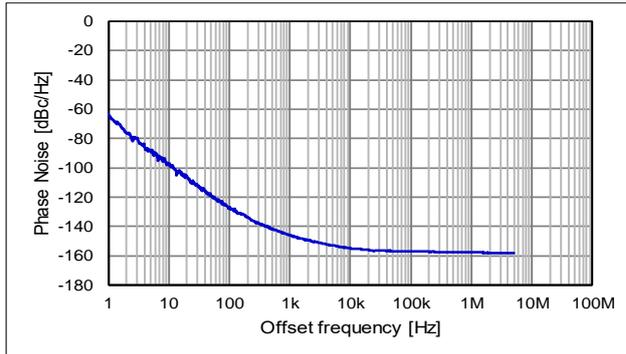
Phase Jitter (Offset frequency: 12 kHz to 5 MHz)
