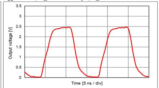
$V_{CC} = 1.8 \text{ V}$ ,  $L_{CMOS} = 15 \text{ pF}$ ,  $T_{use} = +25 \text{ }^\circ\text{C}$
