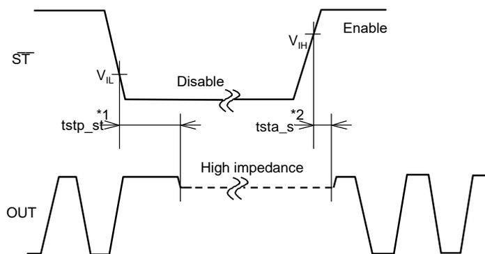
\*1 The period from  $\overline{ST} = V_{IL}$  to  $OUT = \text{High impedance (Disable)}$
