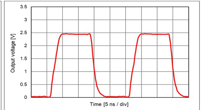
V<sub>CC</sub> = 1.8 V, L<sub>CMOS</sub> = 15 pF, T<sub>use</sub> = +25 °C
