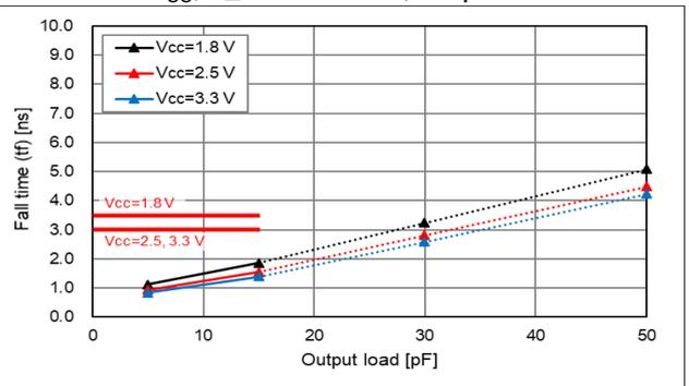
10% - 90% V<sub>CC</sub>, L<sub>CMOS</sub> = 15 pF, Temp. Char.
