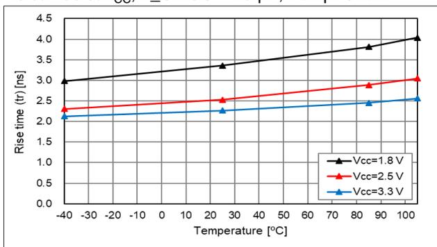
10% - 90% V<sub>CC</sub>, T<sub>use</sub> = +25 °C, Output load Char.
