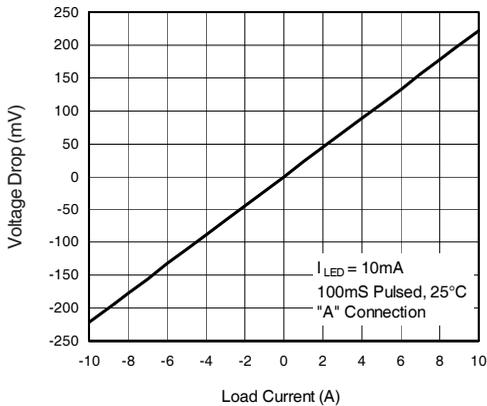
Figure 3. Linearity Characteristics
