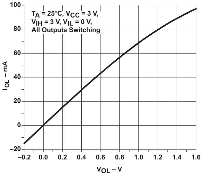
Figure 5. Output Drive Current (I<sub>OL</sub>) vs LOW-level Output Voltage (V<sub>OL</sub>)
