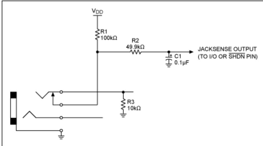
Figure 1. Jack-sensing circuit.
