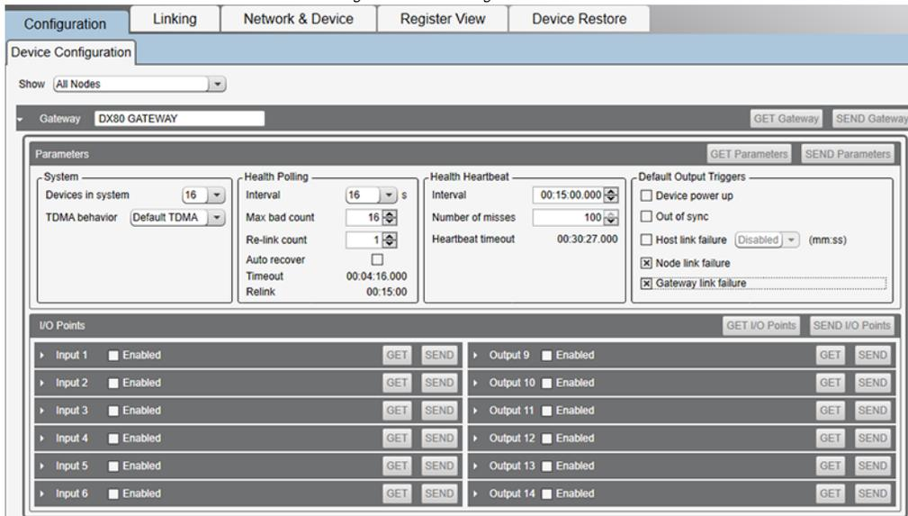
Use a USB to RS-485 adapter cable to connect a standalone DX80 Gateway to the computer. For DXM Controllers with an internal DX80 radio, connect a computer to the DXM Controller using the supplied USB or Ethernet connection. Download the most recent revisions of the configuration software from Banner Engineering's website: <https://www.bannerengineering.com/us/en/products/wireless-sensor-networks/reference-library/software.html>.
