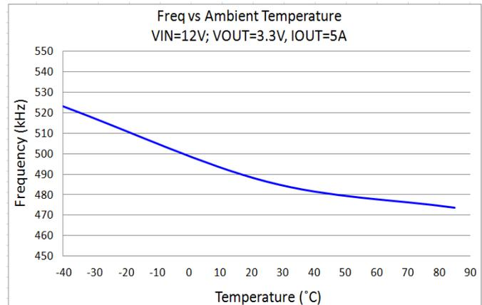
**Typical Performance Characteristics** (cont.) (@ $T_A = +25^\circ\text{C}$ ,  $V_{IN} = 12\text{V}$ ,  $V_{OUT} = 3.3\text{V}$ , unless otherwise specified.)
