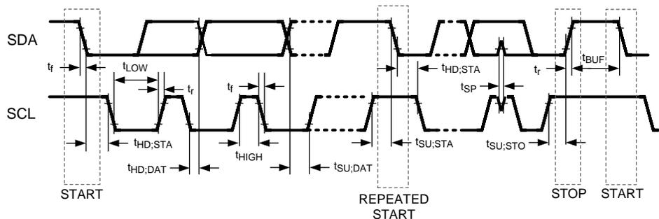
Figure 1. I<sup>2</sup>C Timing
