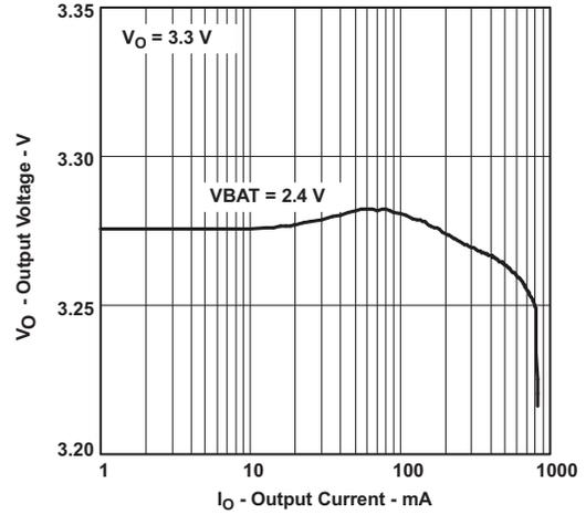
Figure 6. TPS61025 Output Voltage vs Output Current
