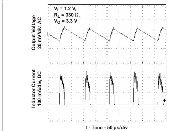
Figure 18. TPS61025 Output Voltage In Power Save Mode
