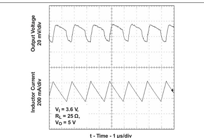
Figure 17. TPS61027 Output Voltage In Continuous Mode
