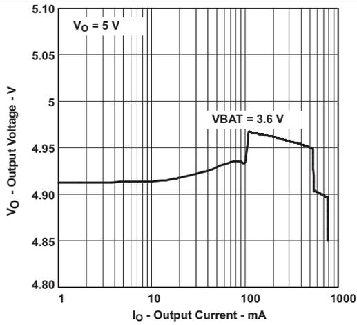
Figure 7. TPS61027 Output Voltage vs Output Current
