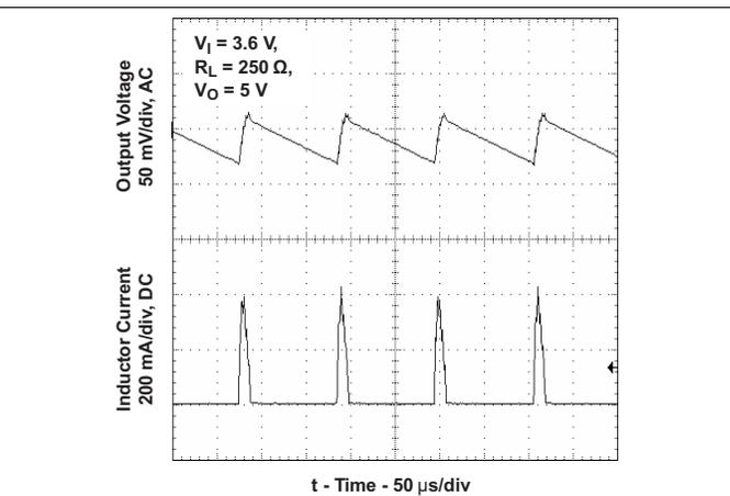
Figure 19. TPS61027 Output Voltage In Power Save Mode
