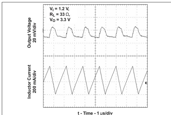
Figure 16. TPS61025 Output Voltage In Continuous Mode
