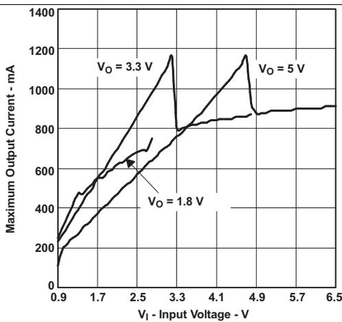
Figure 1. Maximum Output Current vs Input Voltage
