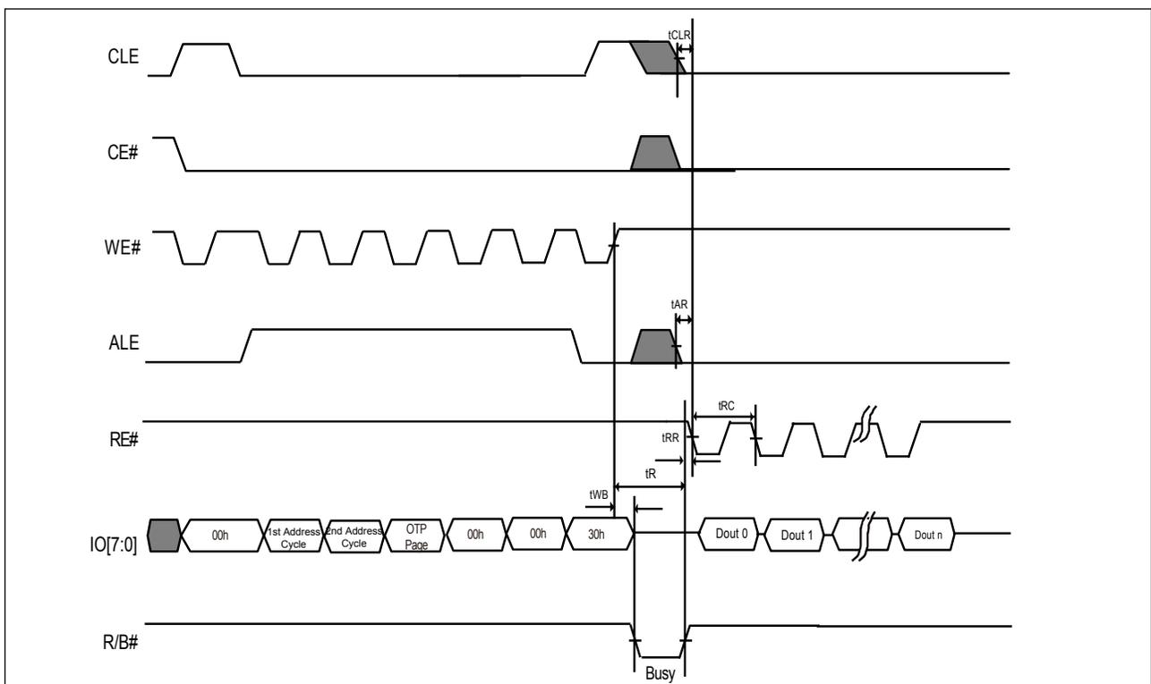
Figure 30. AC Waveforms for OTP Data Read with Random Data Output
