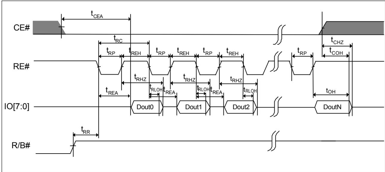
**Figure 10. AC Waveforms for Random Data Output**
