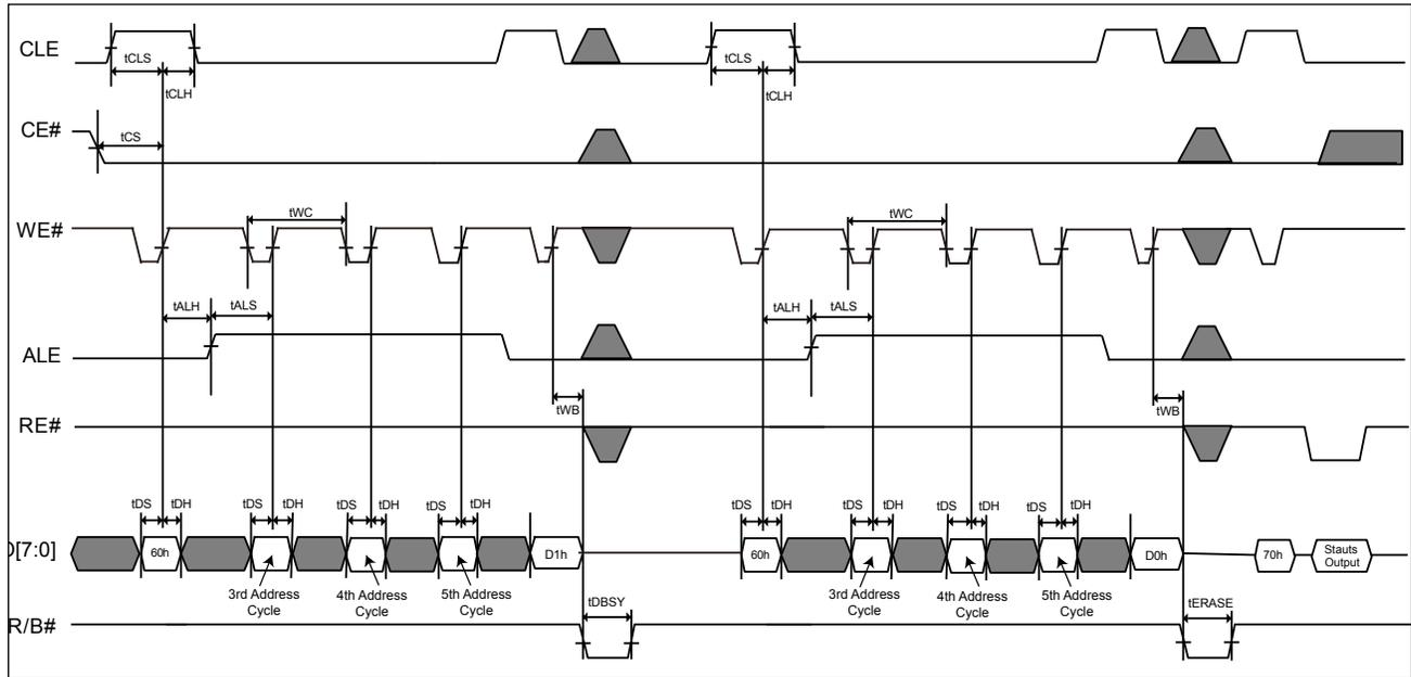
**Figure 38. AC waveforms for Two-plane Program (Traditional)**
