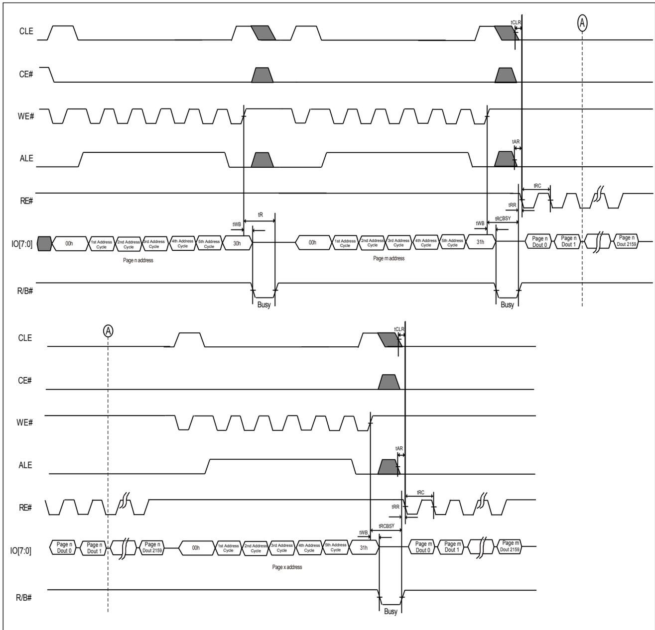
Figure 13. AC Waveforms for Random Data In (For Page Program)
