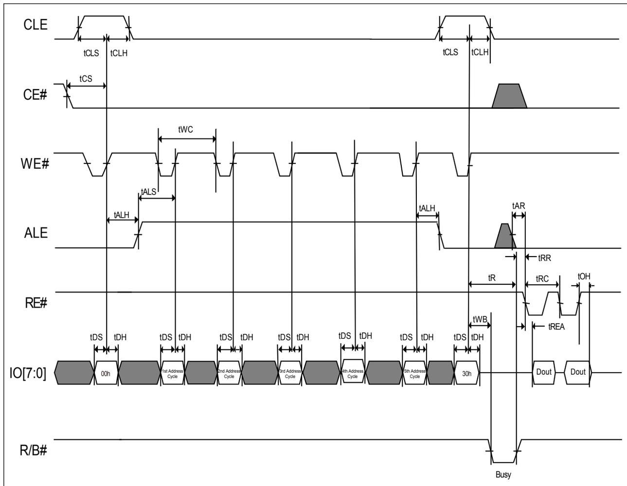
Figure 7. AC Waveforms for Read Operation (Intercepted by CE#)
