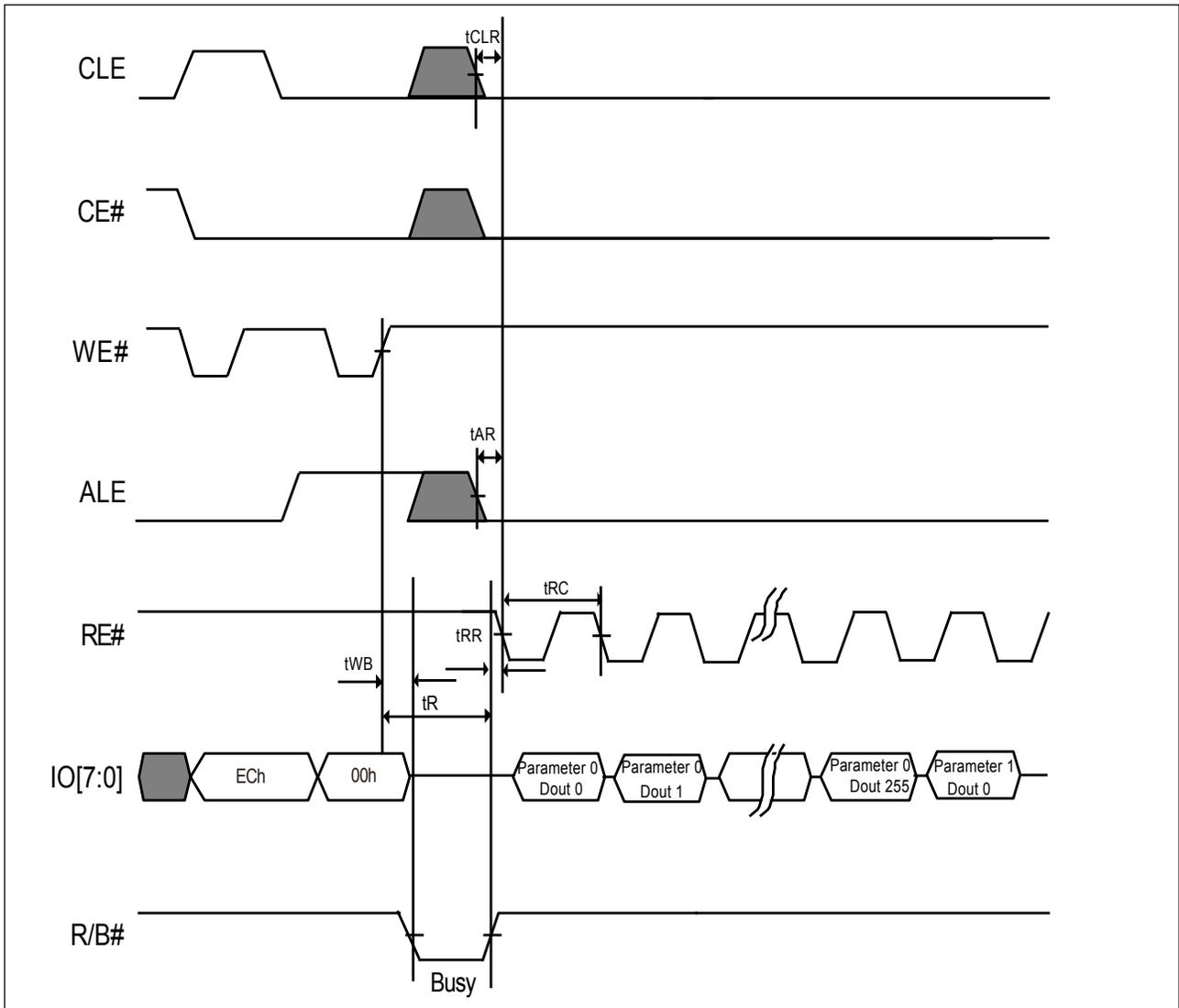
Figure 24. AC Waveforms for Parameter Page Read (ONFI) Random Operation (For 05h-E0h)
