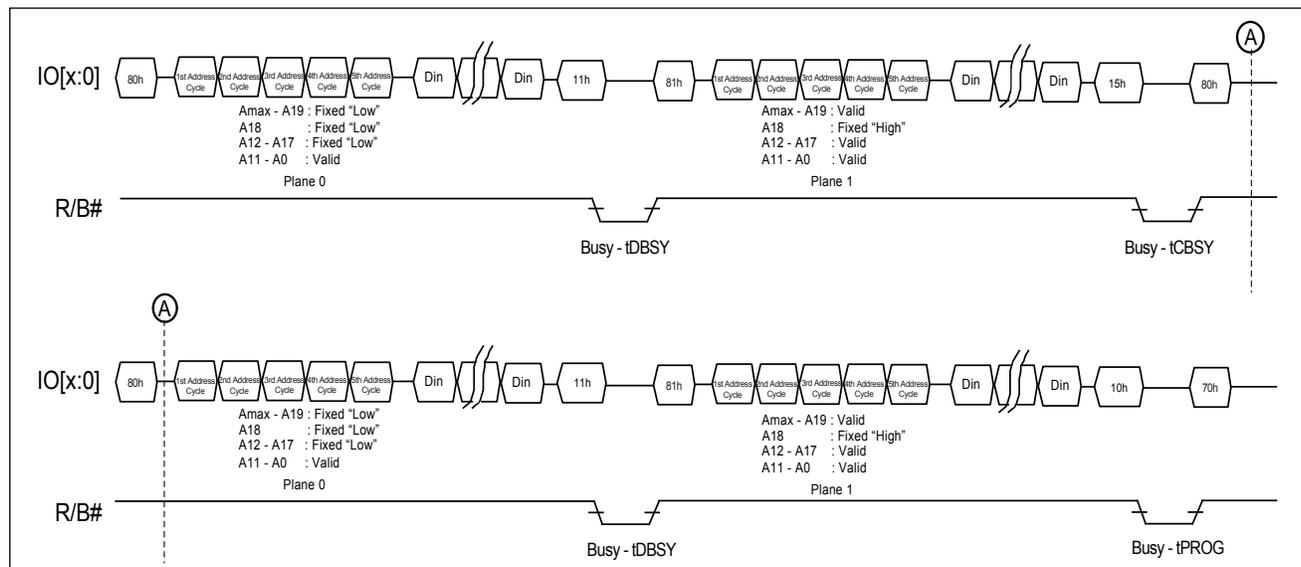
**Figure 40. AC waveforms for Two-plane Erase (Traditional)**
