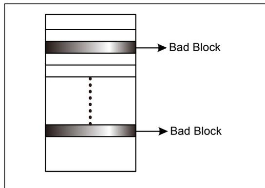
While the device is shipped, the value of all data bytes of the good blocks are FFh. The 1st byte of the 1st and 2nd page in the spare area for bad block will be 00h. The erase operation at the bad blocks is not recommended.
