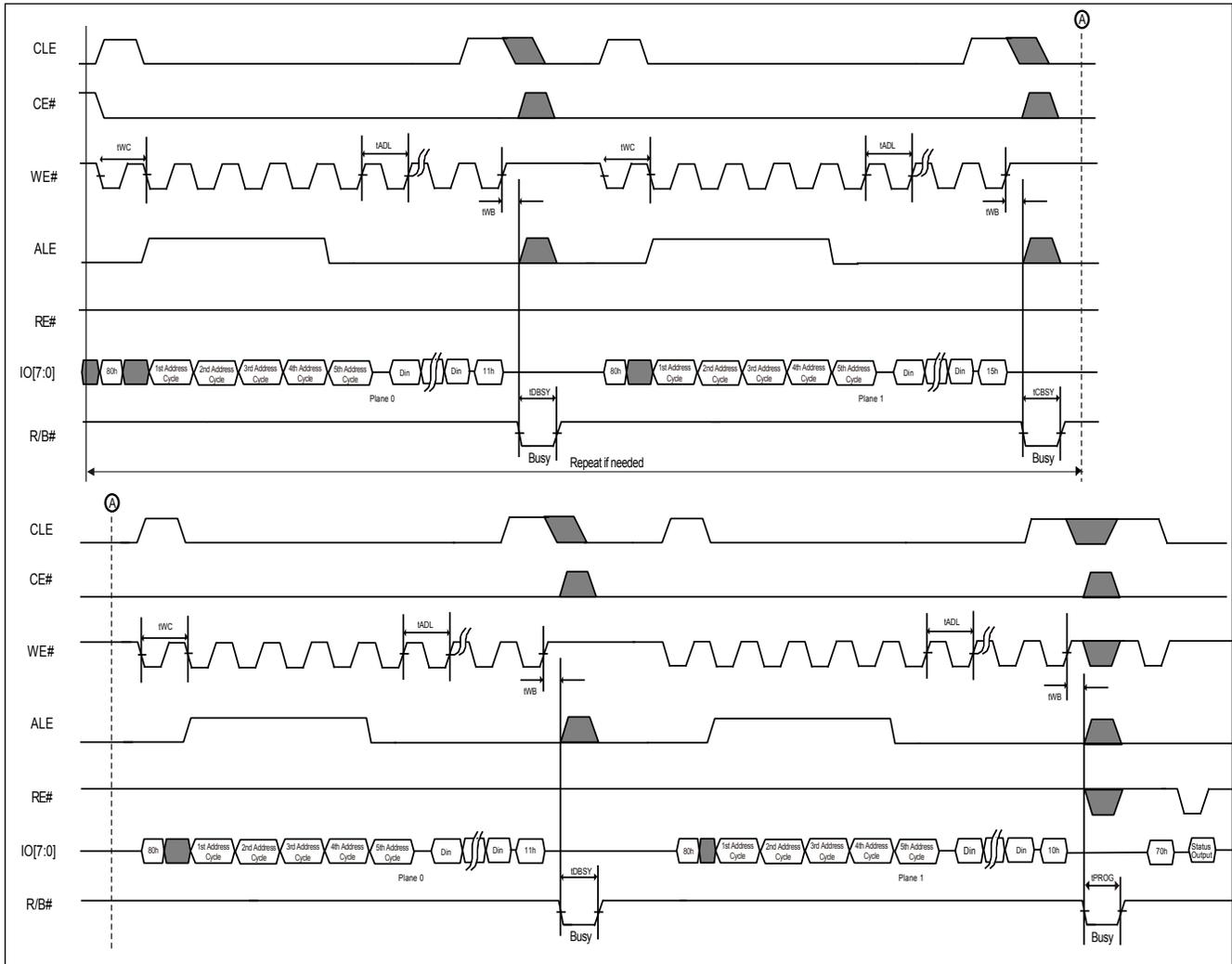
**Figure 37. AC Waveforms for Two-plane Erase (ONFI)**
