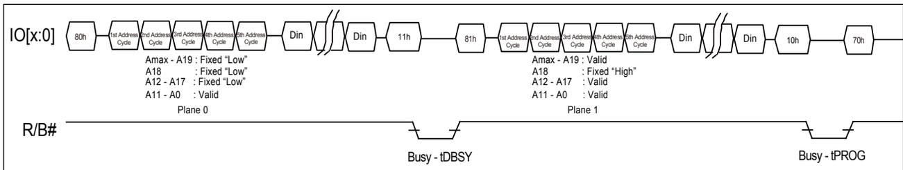
**Figure 39. AC waveforms for Two-plane Cache Program (Traditional)**
