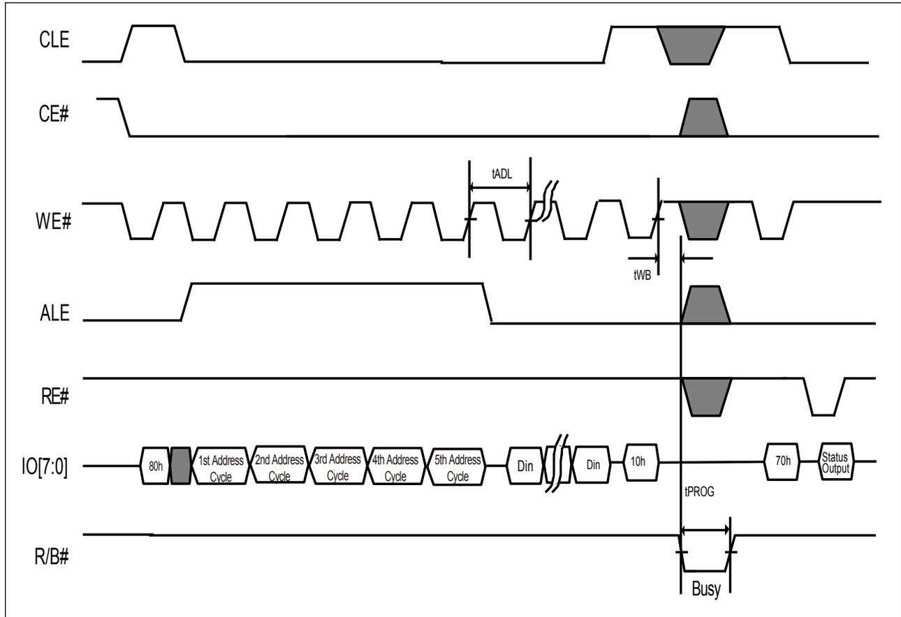
Figure 32. AC Waveforms for OTP Data Program with Random Data Input
