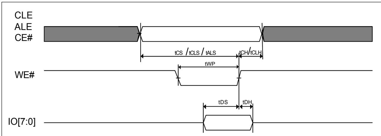
Figure 3. AC Waveforms for Address Input Cycle
