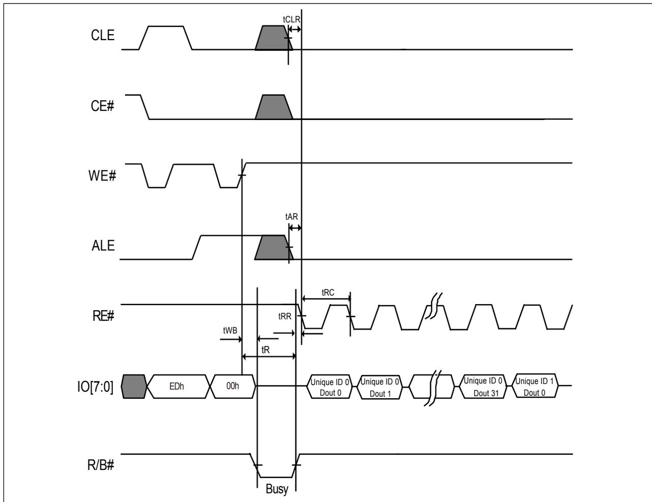
Figure 26. AC waveforms for Unique ID Read Operation (For 05h-E0h)
