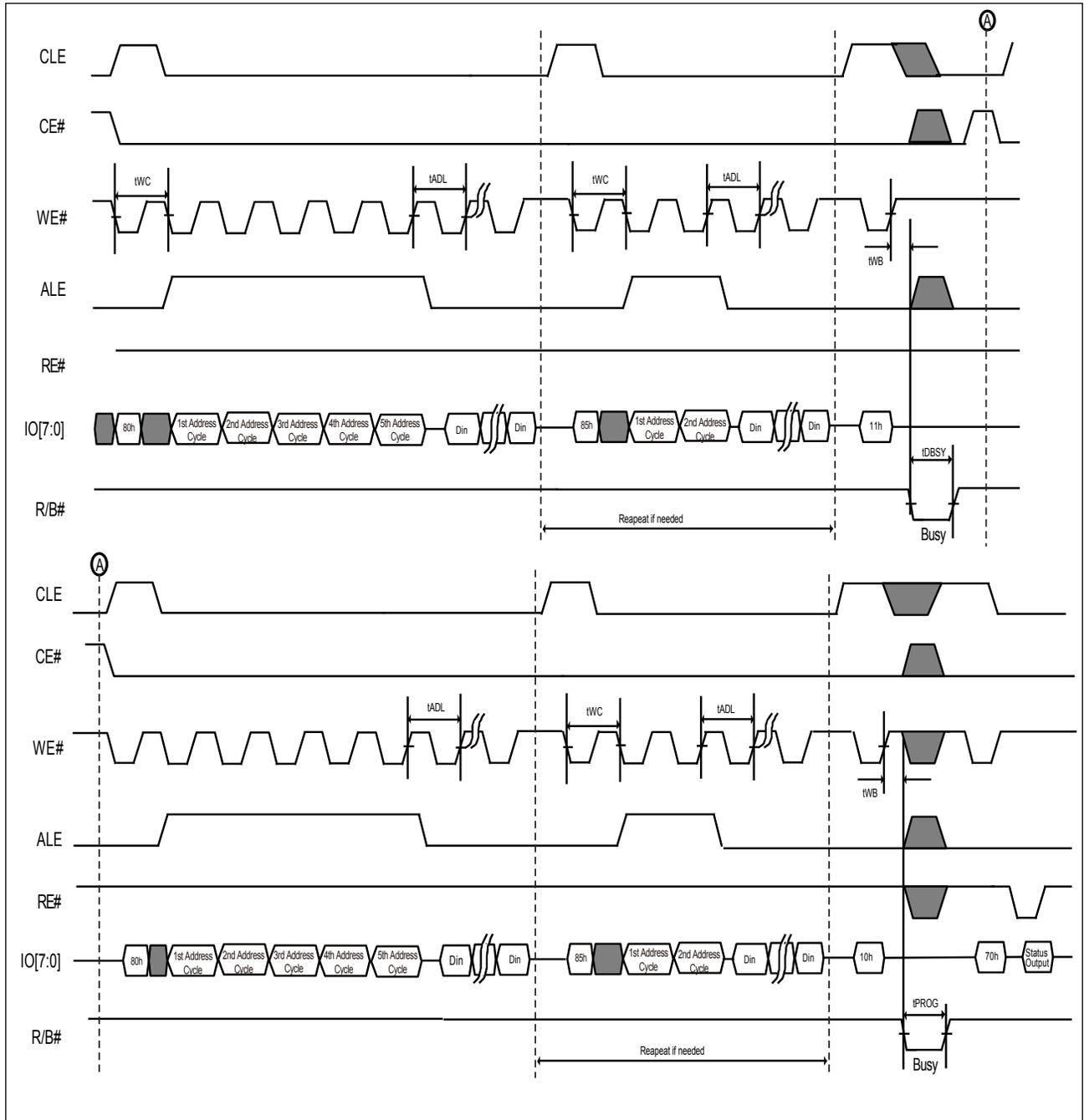
Figure 36. AC Waveforms for Two-plane Cache Program (ONFI)
