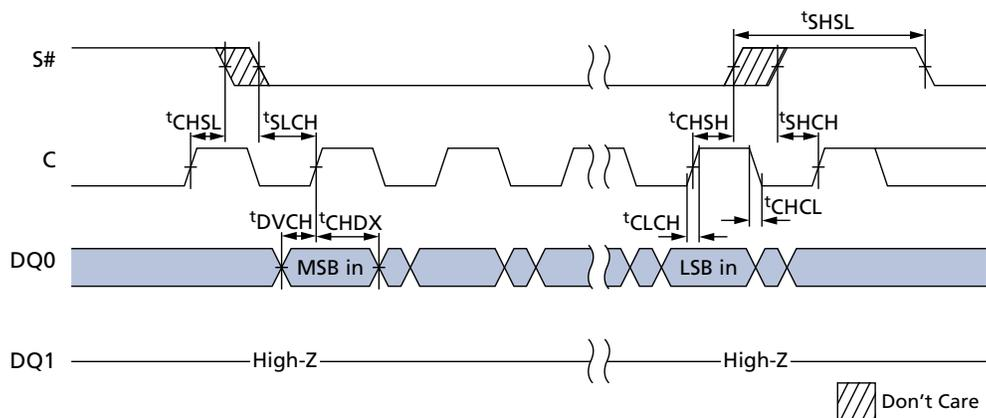
Figure 55: Serial Input Timing DTR
