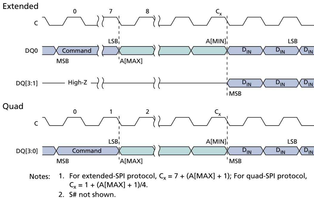
**Figure 41: EXTENDED QUAD INPUT FAST PROGRAM Command**
