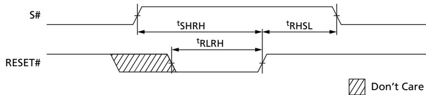
**Figure 53: Reset Enable and Reset Memory Timing**
