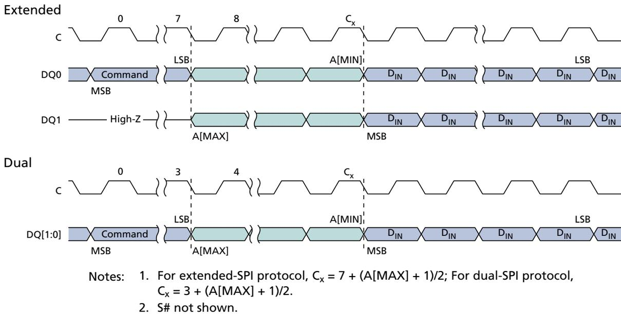
**Figure 40: QUAD INPUT FAST PROGRAM Command**
