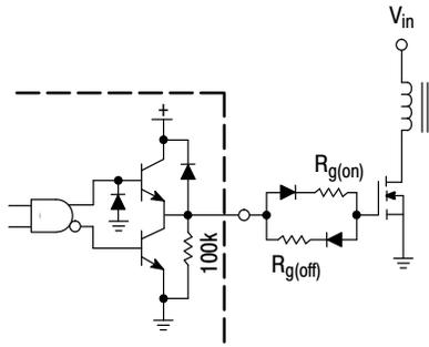
In noise sensitive applications, both conducted and radiated EMI can be reduced significantly by controlling the MOSFET's turn-on and turn-off times.
