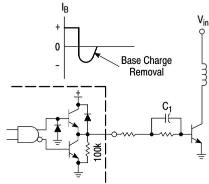
The totem-pole outputs can furnish negative base current for enhanced transistor turn-off, with the addition of capacitor C<sub>1</sub>.
