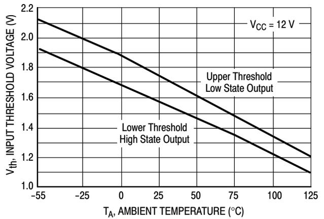
Figure 5. Logic Input Threshold Voltage versus Temperature
