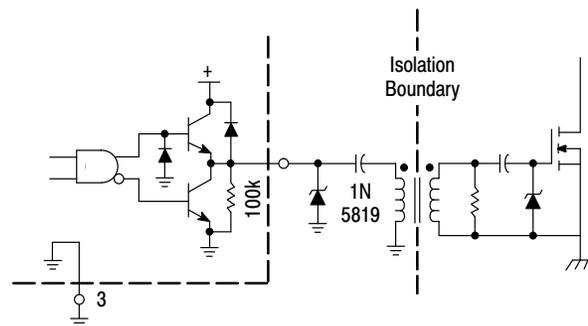
Figure 22. Isolated MOSFET Drive
