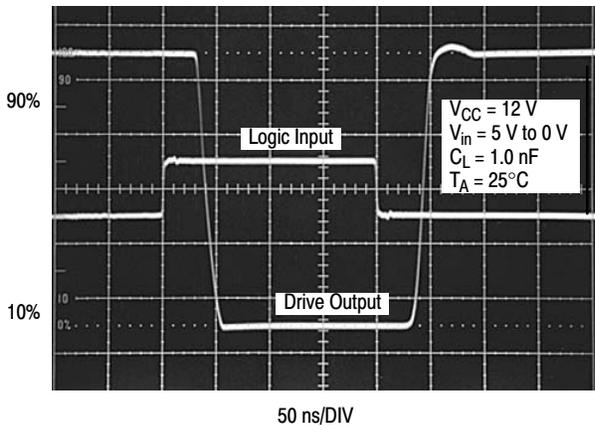
Figure 8. Propagation Delay
