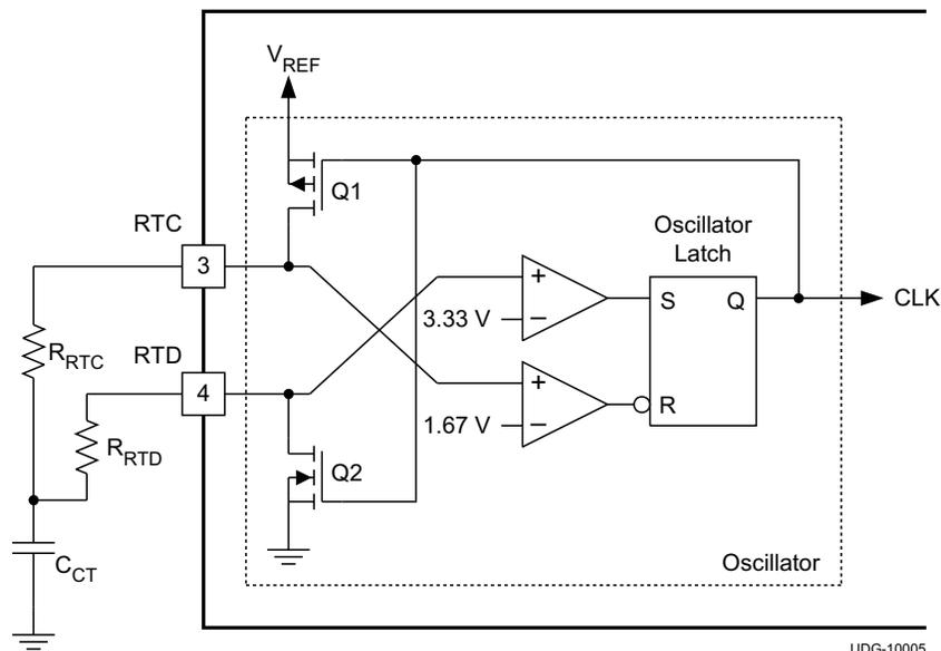
**Figure 1. Oscillator Function**
