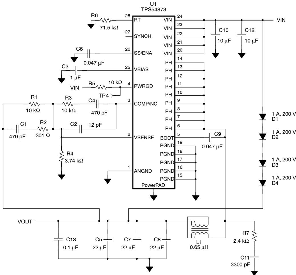
**Figure 9. Application Circuit**
