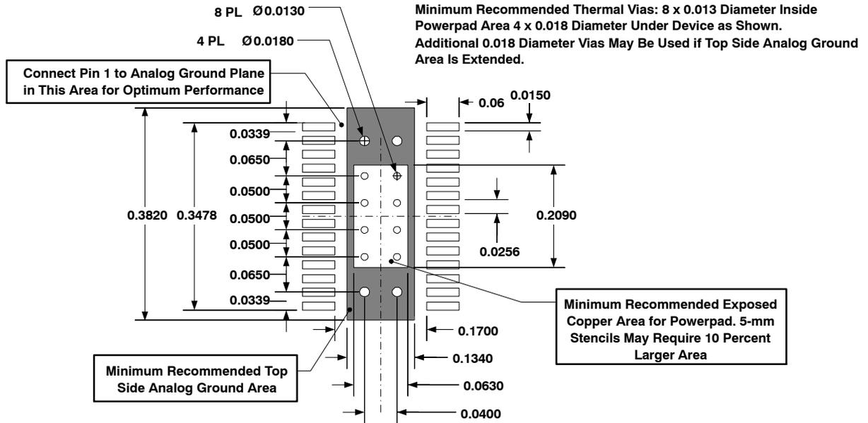
Figure 11. Recommended Land Pattern for 28-Pin PWP PowerPAD
