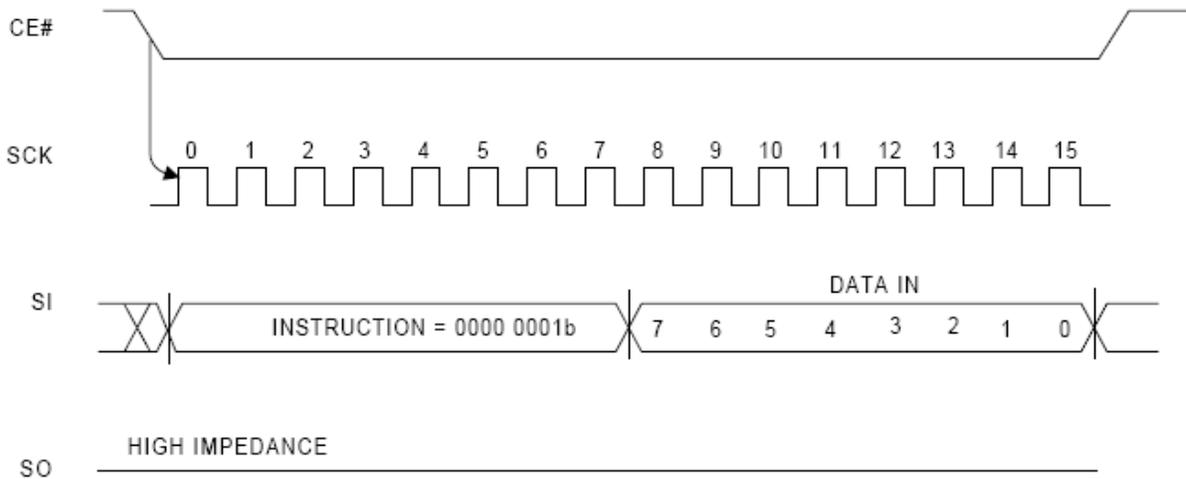
**Figure 11. Write Status Register Sequence**
