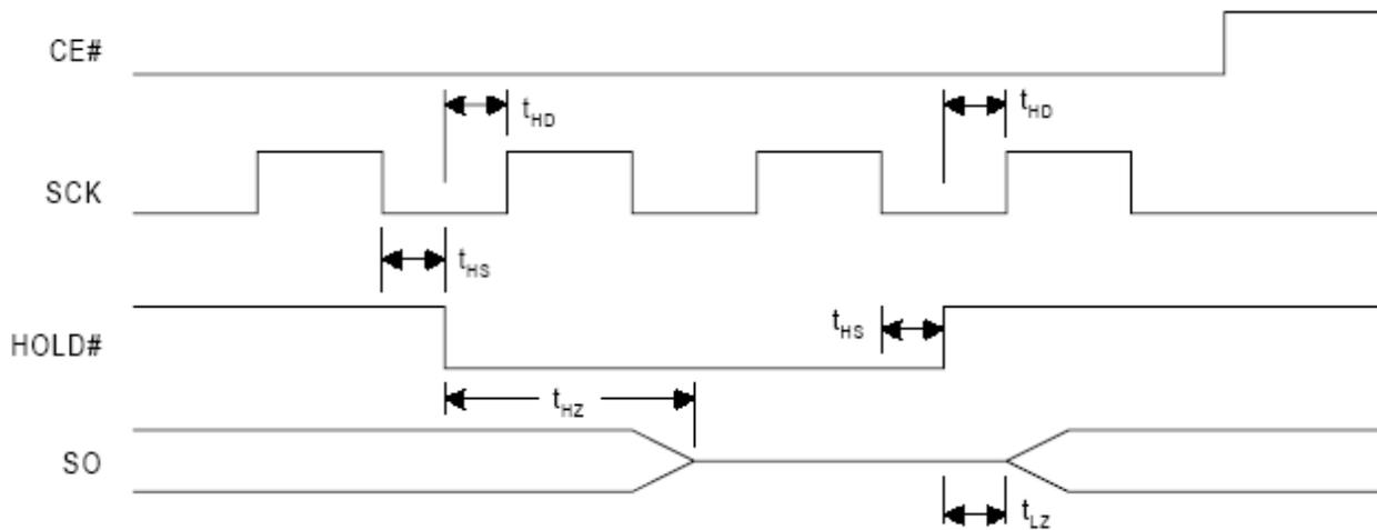
Figure 2. HOLD Timing Diagram
