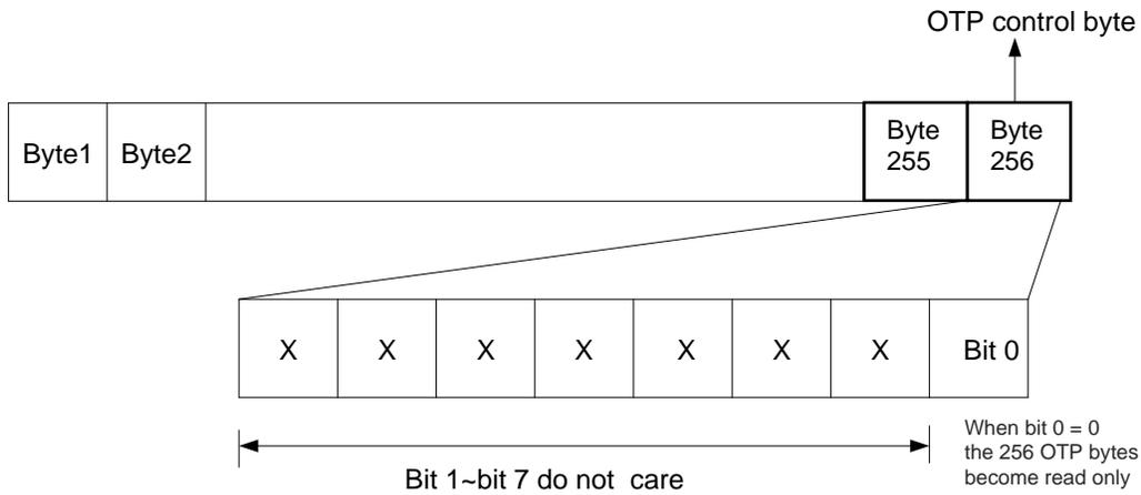
Figure 27. Control Byte to lock security memory
