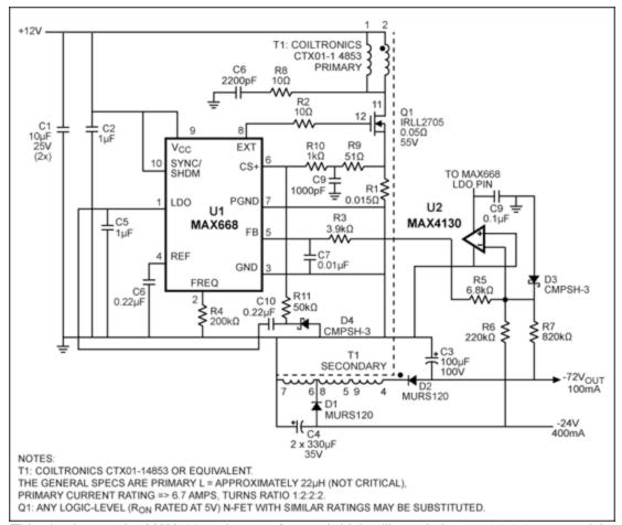
This circuit uses the MAX668 and a transformer (which will need about a 1:2:2:2 turns ratio) to make a flyback converter. The op amp inverts the feedback from both negative output voltages.
