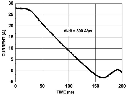
Figure 14. FDMS7658AS SyncFET™ Body Diode Reverse Recovery Characteristic
