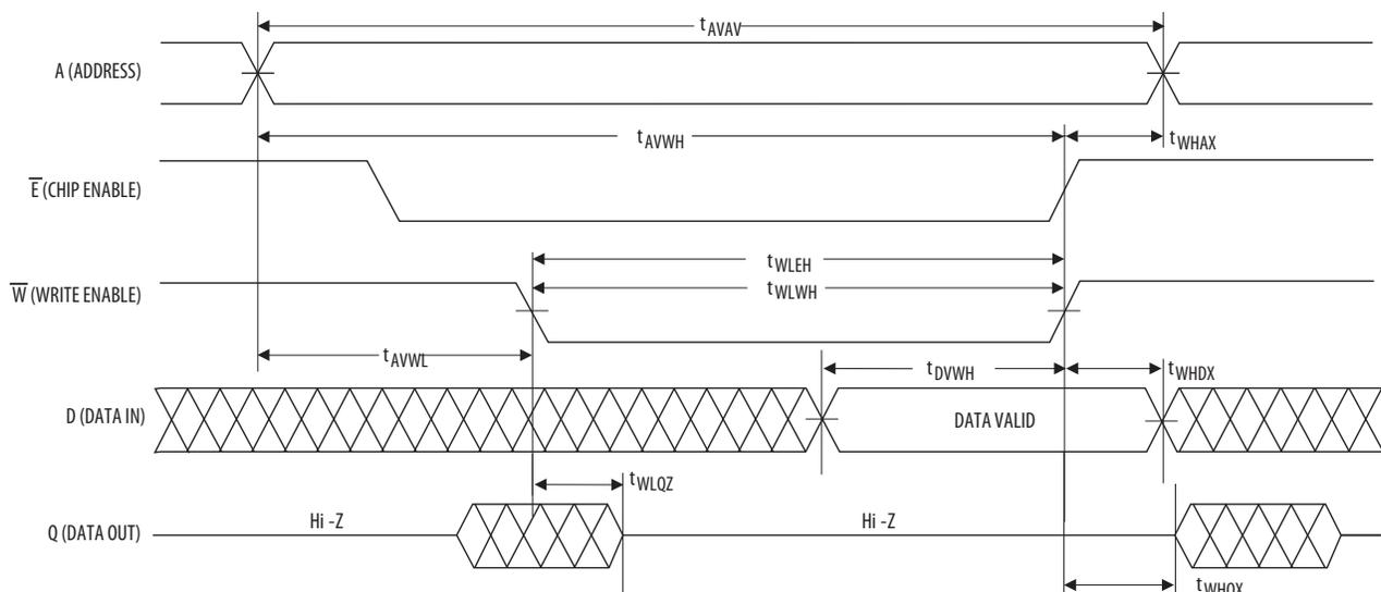
Table 3.5 Write Cycle Timing 2 ( $\bar{E}$  Controlled) <sup>1</sup>
