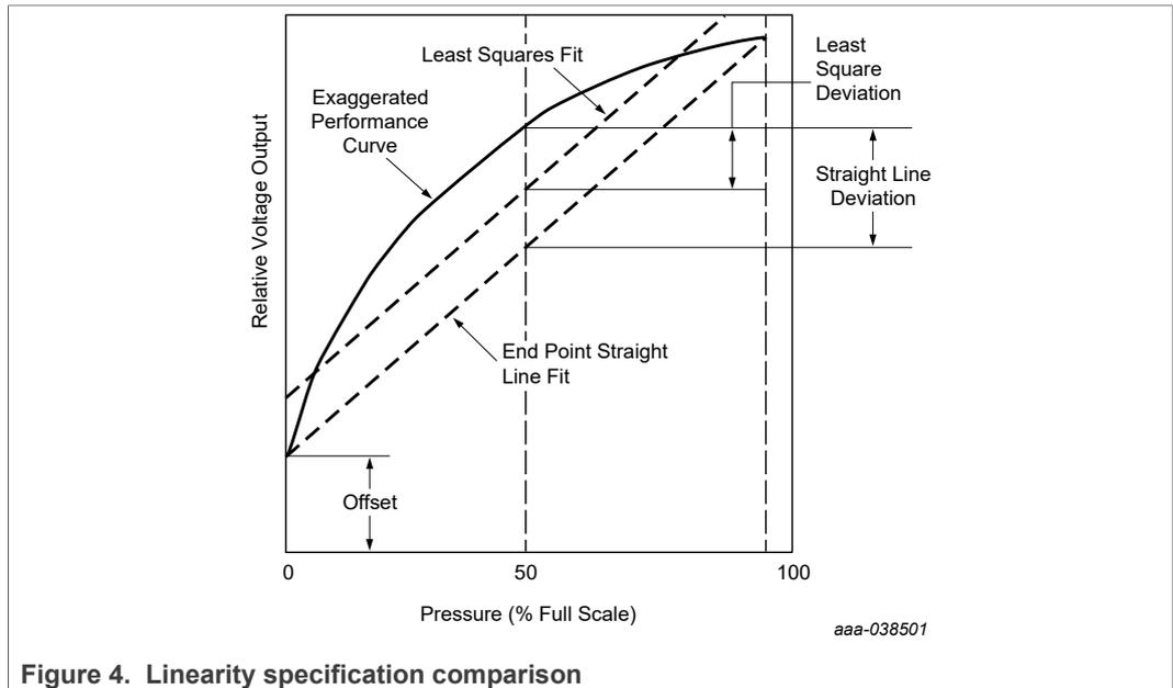
Figure 4. Linearity specification comparison
