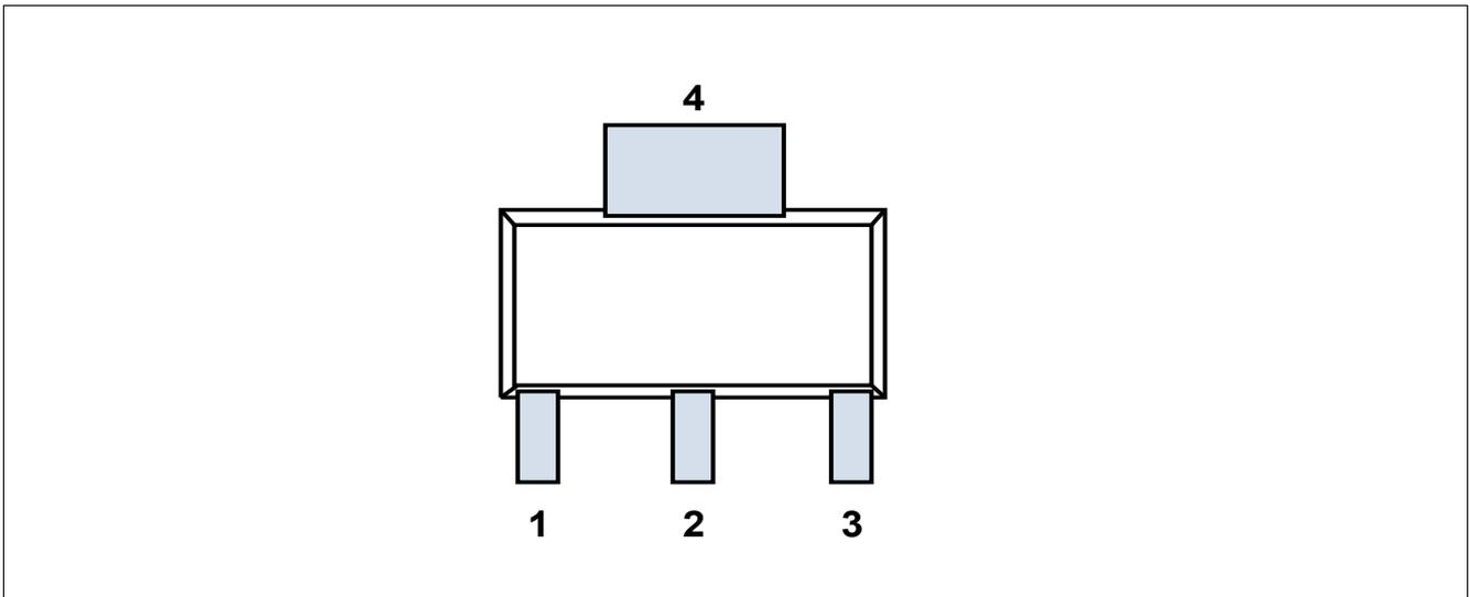
Figure 3 Pin configuration top view, SOT-223-4
