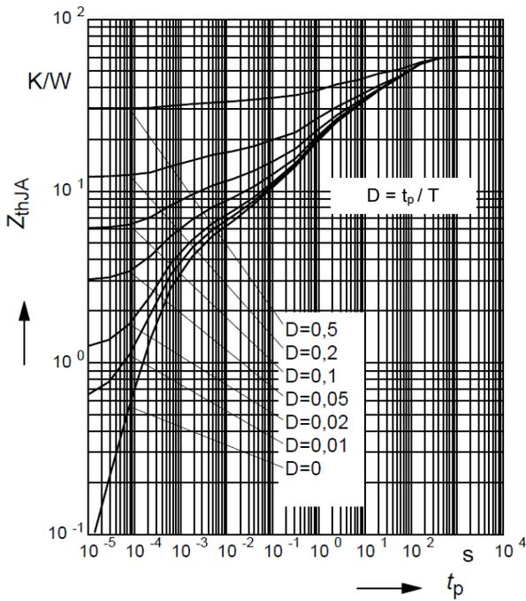
Transient Thermal Impedance  $Z_{thJA}$  versus Pulse Time  $t_p$  @ min footprint
