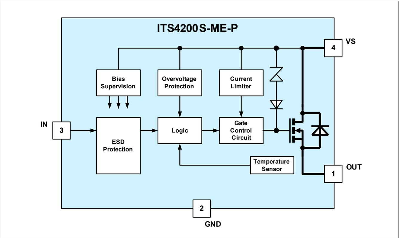
Figure 1 Block diagram
