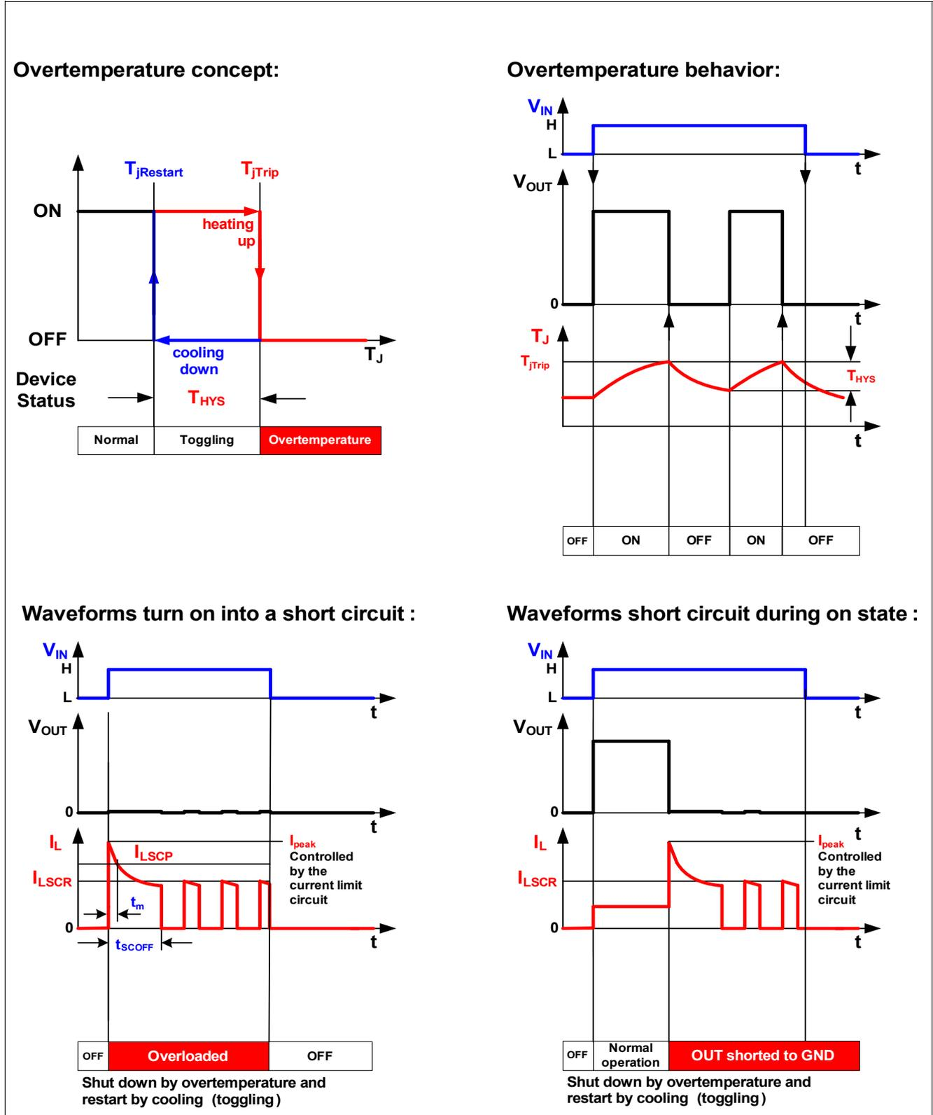
Figure 7 Protective behaviour of the ITS4200S-ME-P
