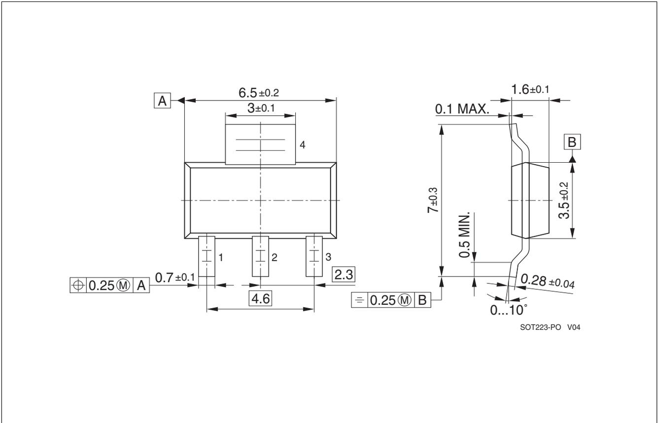
**Figure 8** SOT-223-4 (Plastic Dual Small Outline Package, RoHS-Compliant)
