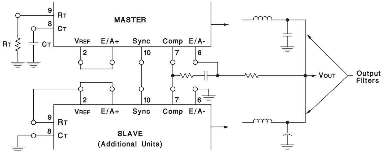
Slaving allows parallel operation of two or more units with equal current sharing.
