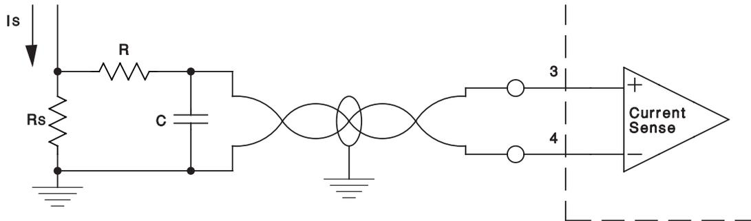
A small RC filter may be required in some applications to reduce switch transients.
