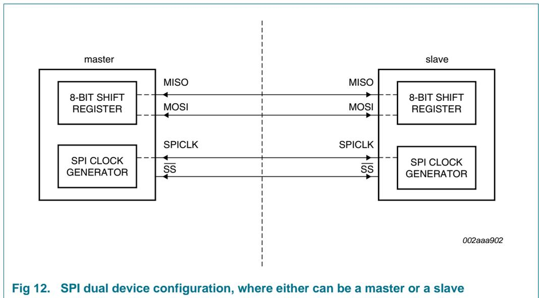
Fig 12. SPI dual device configuration, where either can be a master or a slave
