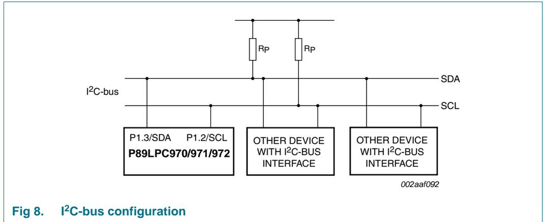
**Fig 8.** I<sup>2</sup>C-bus configuration
