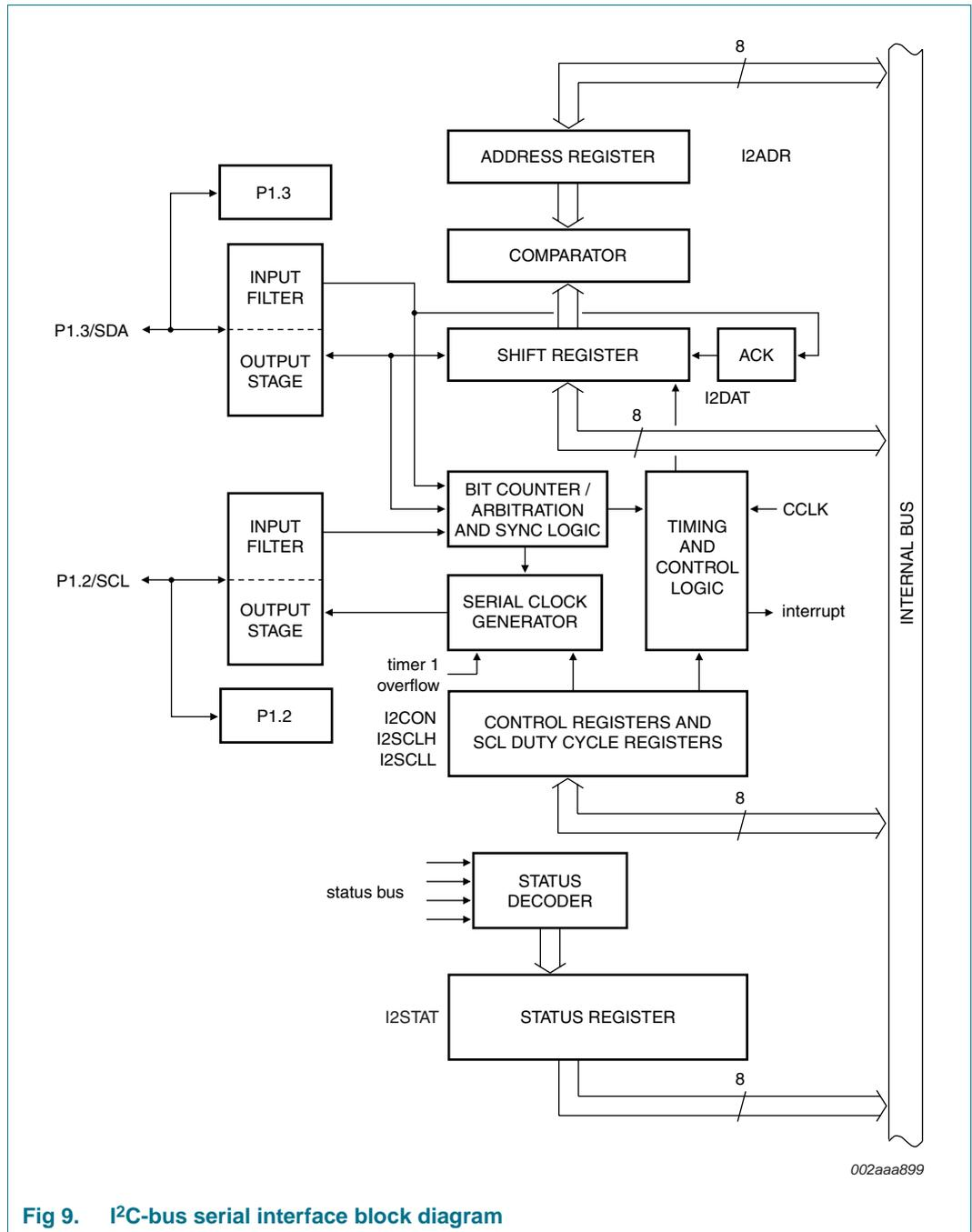
**Fig 9. I<sup>2</sup>C-bus serial interface block diagram**
