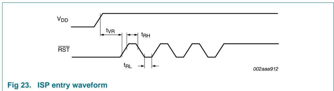
Fig 23. ISP entry waveform
