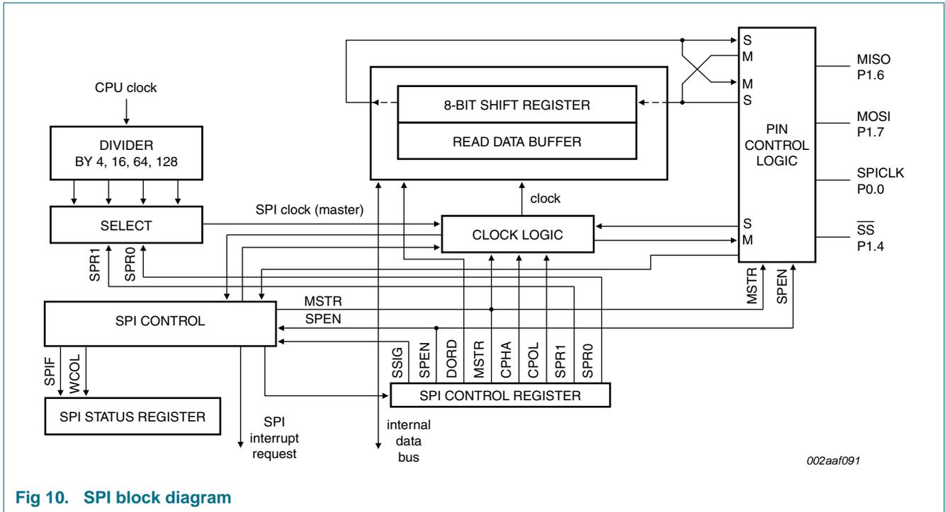
Fig 10. SPI block diagram
