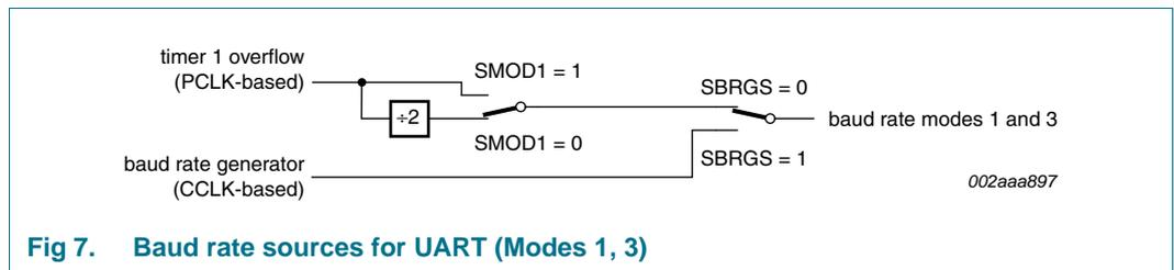
**Fig 7. Baud rate sources for UART (Modes 1, 3)**
