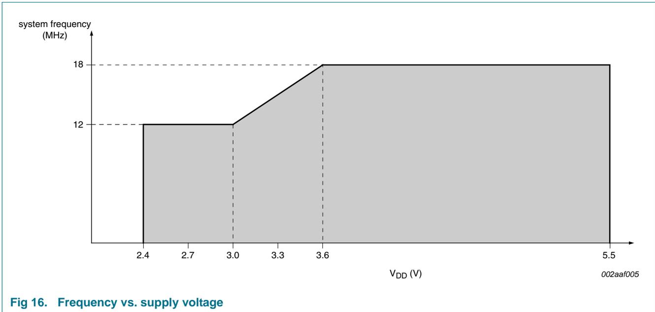
Fig 16. Frequency vs. supply voltage
