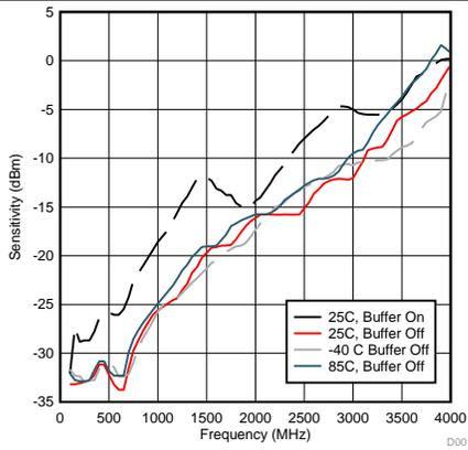
Figure 10. Sensitivity for External VCO Input (Fin) Pin
