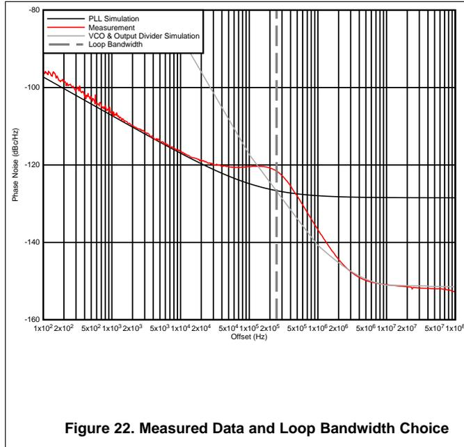
Figure 22. Measured Data and Loop Bandwidth Choice
