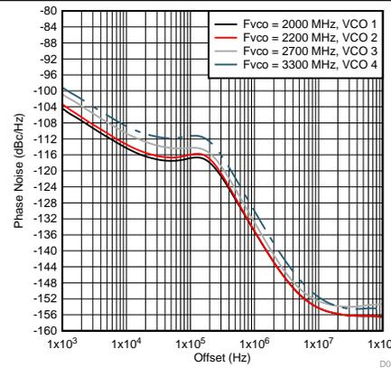
Figure 5. Closed Loop Noise for Wider Bandwidth
