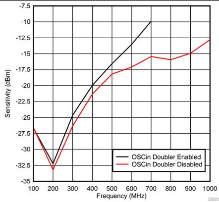
Figure 12. OSCin Input Sensitivity
