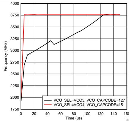
Figure 7. VCO Digital Calibration Time
