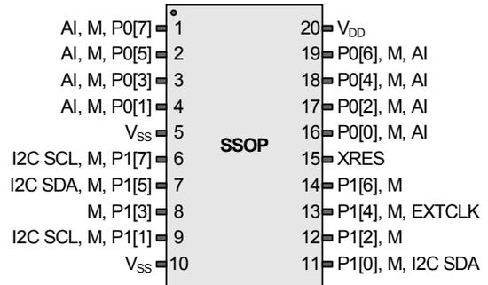
LEGEND A = Analog, I = Input, O = Output, and M = Analog Mux Input.
